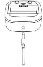
Connect the sensor cable to the bottom of the water sensor.
