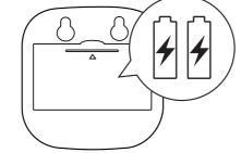
Remove the battery cover by gently pressing down on the tab.
