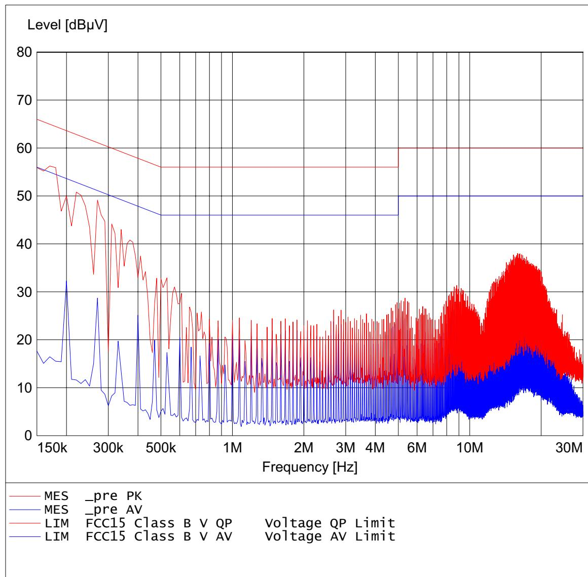
**EMI voltage test in the ac-mains according to FCC Part 15**
