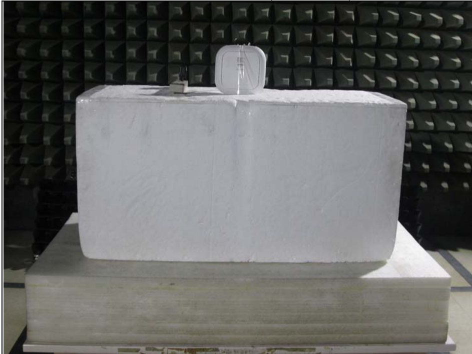
Radiated Emission Test (Above 1GHz)
