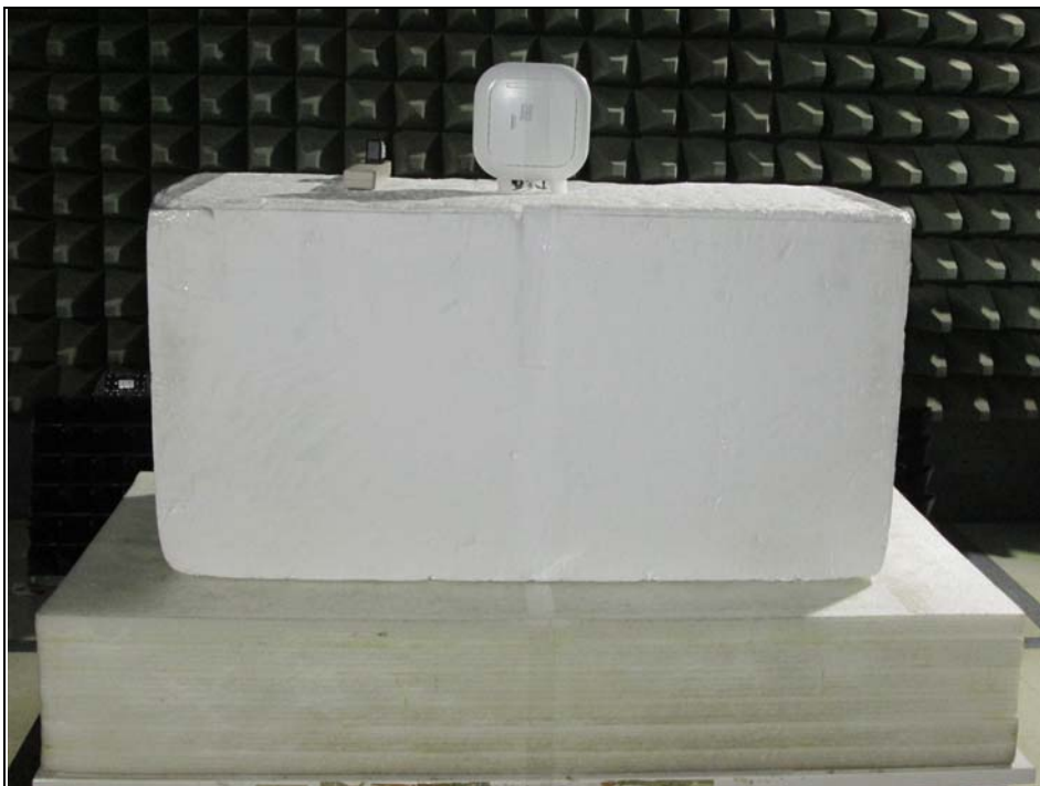
Radiated Emission Test (Above 1GHz)
