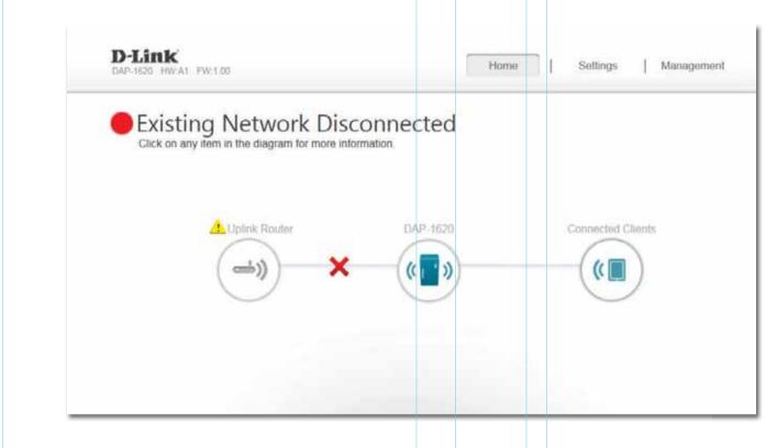
Uplink Router: This icon shows the status of the Internet connection to the uplink router. It is grey if the DAP-1620 is not connected to an uplink router. Once connected, click on it to see its connection details.
