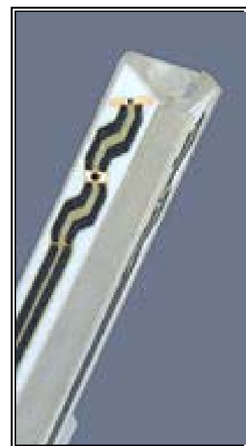
Inside View of ET3DV6 E-field Probe
