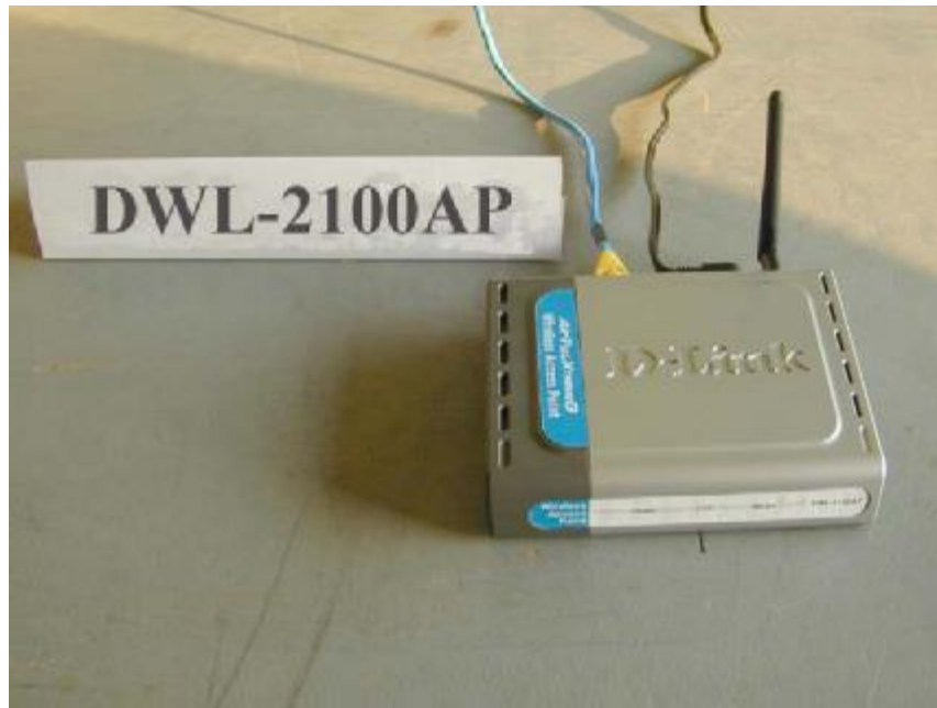
Photo 3: Radiated Emission Test Set-up
