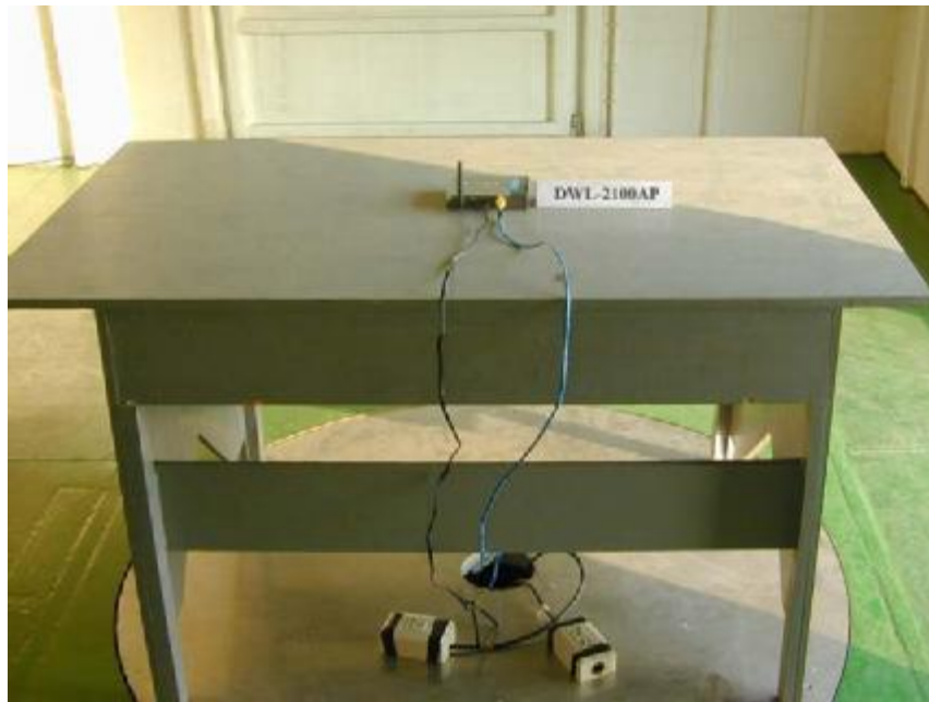
Photo 2: Radiated Emission Test Set-up
