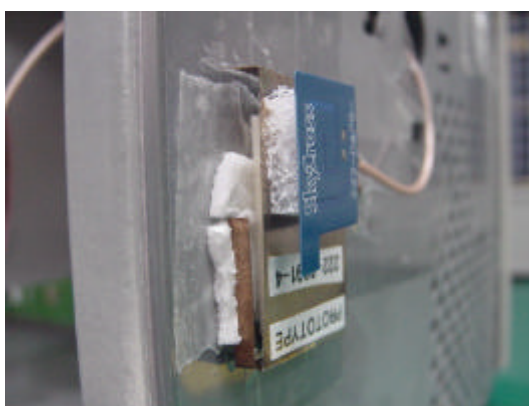
Figure 2: Two Types of Internal Antennas
