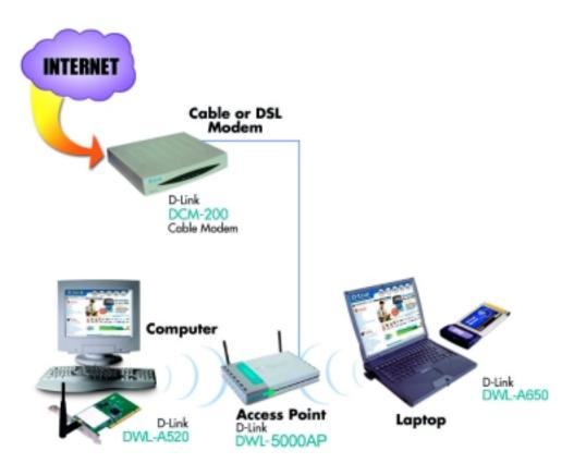
Please note that this type of installation requires that your ISP (Internet Service Provider) provides you a static IP address for each computer and the Access Point on your network. Please refer to the manual that came with your Access Point to determine its configuration.
