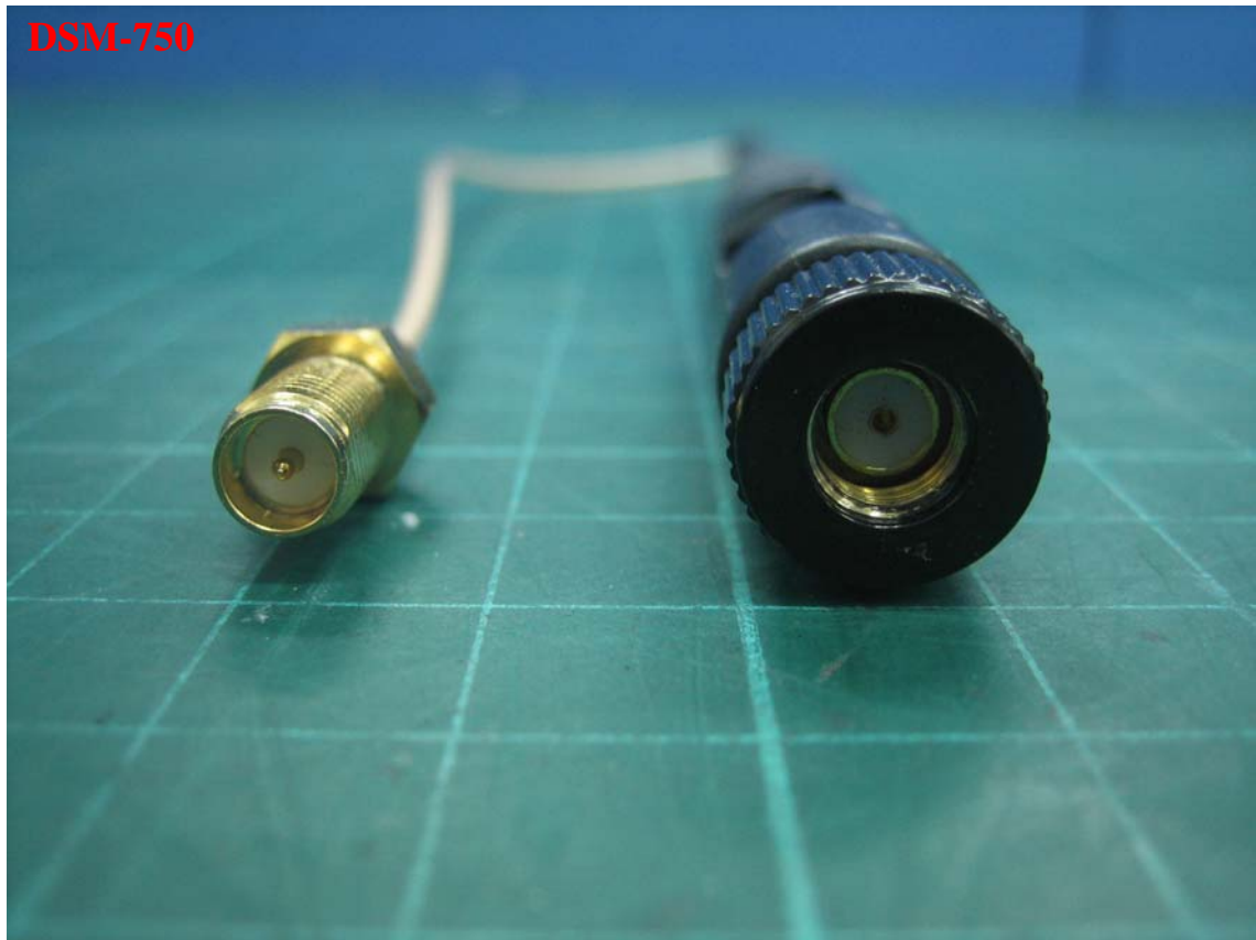
Photo 4: External photo of Antenna
