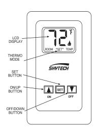
The wall/transmitter operates on (2) 3V Button Cell (Included) which powers the LCD screen. These batteries are made specifically for remote controls and electronic lighters. Before using the transmitter the 3V batteries must be installed into the battery compartments.
