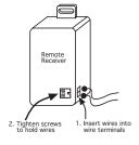
A qualified electrician or a gas technician who is familiar with the gas appliance and gas valves that will be operated by this remote should install this remote control system. Incorrect wiring connections **WILL** cause damage to the gas valve or electronic module operating the gas appliance and may also damage the remote receiver. Attach the two 18 gauge wires provided to the receiver as shown.
