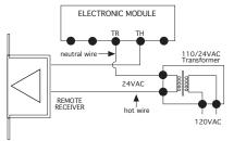
Connect the neutral wire from the 24VAC transformer to the TR (transformer) terminal on the ELECTRONIC MODULE. Connect the hot wire from the 24VAC transformer to either of the wire terminals on the remote receiver. Connect another wire (included) between the other receiver wire terminal and the TH (thermostat) terminal on the ELECTRONIC MODULE.
