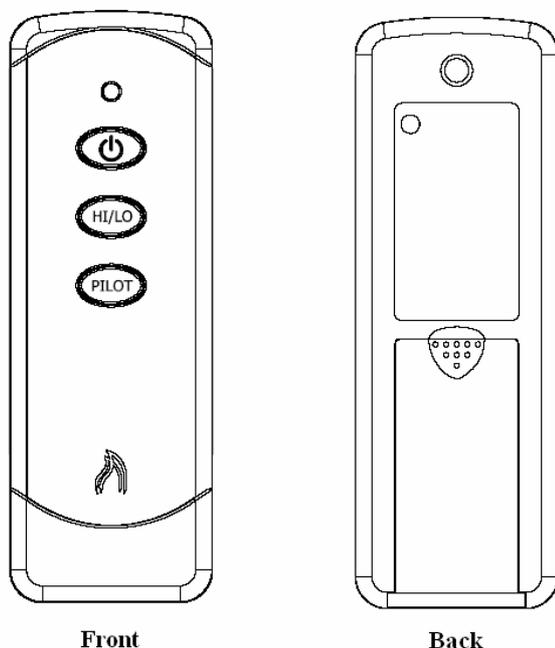
This remote control SYSTEM offers the user a battery-operated remote control that operates most millivolt gas valves used in some heater rated gas logs, gas fireplaces and other gas heating appliances.
