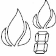
), the main flame indicates burner/valve in operation and additional flame is reserved for specific modulation device.
