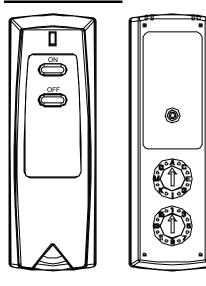
The transmitter operates on a 3v battery (included) made specifically for remote controls and electronic lighters. Before using the transmitter, remove the insulation tab protecting one end of the battery in the battery compartment.
