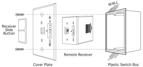
**NOTE:** The remote receiver will only respond to the transmitter when the 3-position slide button on the remote receiver is in the REMOTE position. If the system does not respond to the battery transmitter on initial use, see LEARNING TRANSMITTER TO RECEIVER, and recheck battery positions in the remote receiver.
