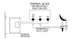
Operation of the remote receiver turns the gas valve ON and OFF based on input signals from the transmitter by pressing the ON/OFF buttons.
