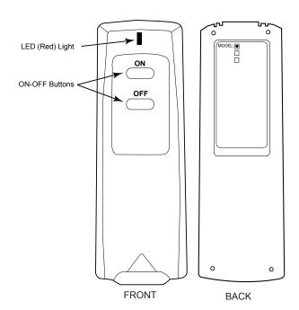
The transmitter is an ON and OFF. There is an LED light that will illuminate when pressing either ON/OFF button. It you do not see the red LED light illuminate check the position of the transmitter's battery.
