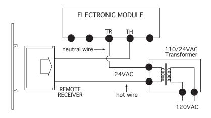
The remote control receiver can be connected, in series, to a 24VAC transformer to the TR (transformer) terminal on the ELECTRONIC MODULE. Connect the hot wire from the 24VAC transformer to either of the wire terminals on the remote receiver. Connect another wire (not included) between the other receiver wire terminal and the TH (thermostat) terminal on the ELECTRONIC MODULE.
