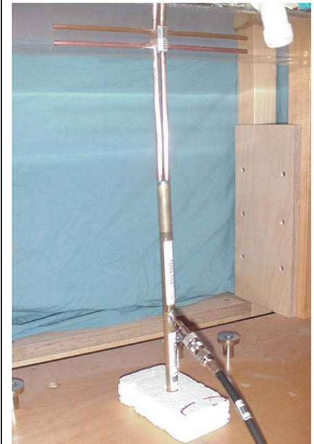
450 MHz Validation Dipole Setup
