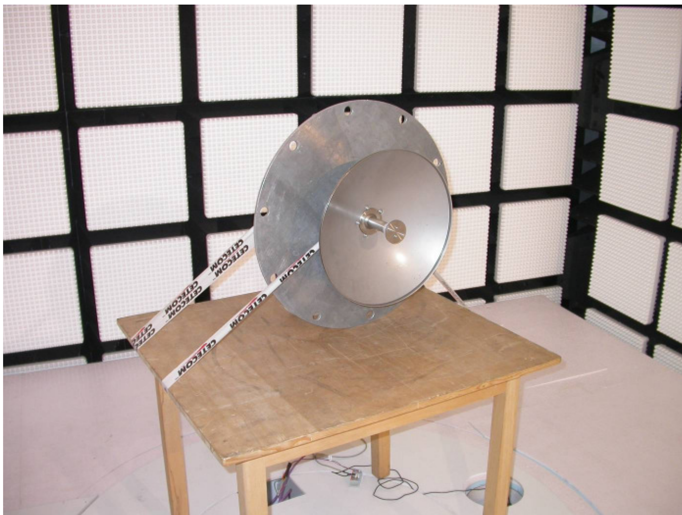
Photo 12 (EUT with parabolic antenna mounted)
