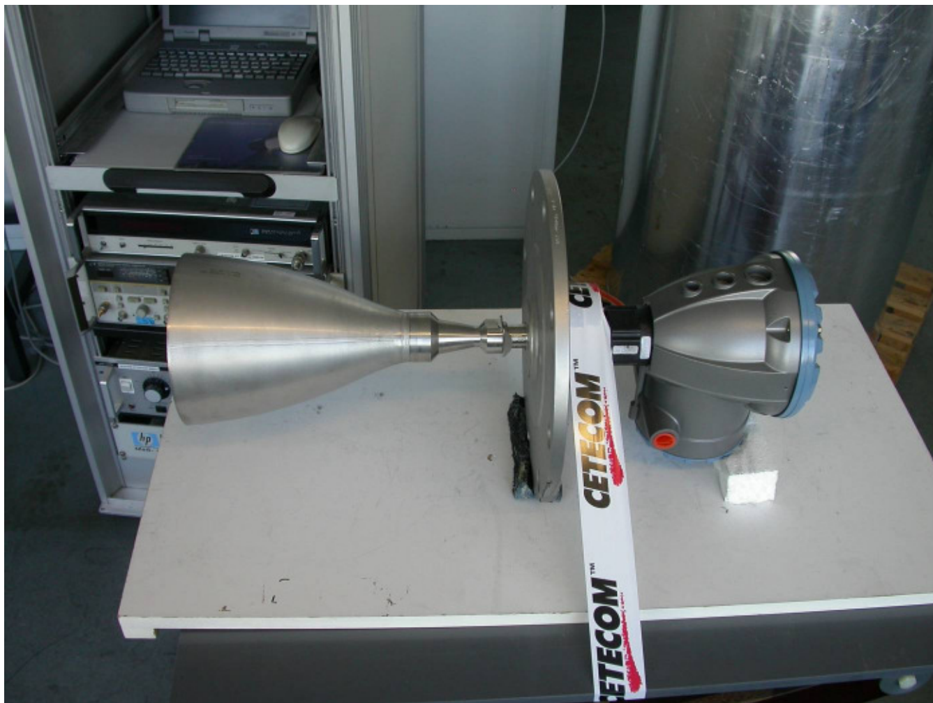
Photo 10 (EUT with horn antenna mounted)
