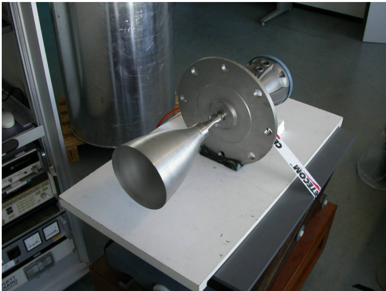
Photo 11 (EUT with horn antenna mounted)
