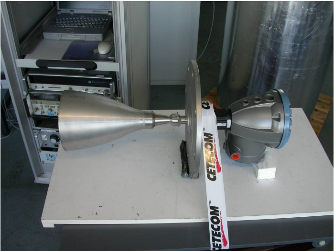
Photo 10 (EUT with horn antenna mounted)
