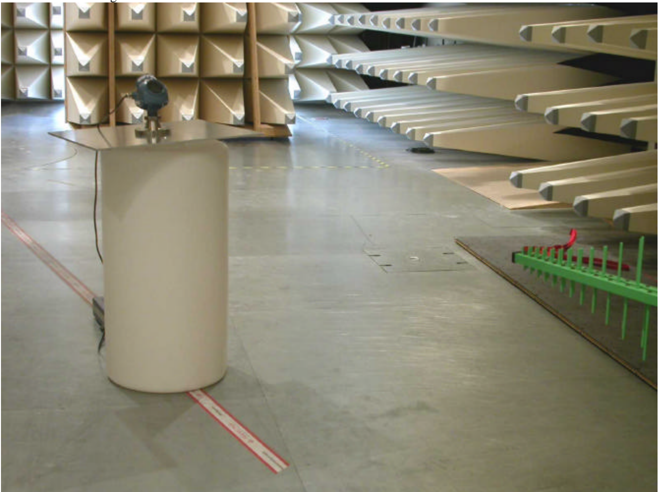
EUT radiating inside a PVC tank
