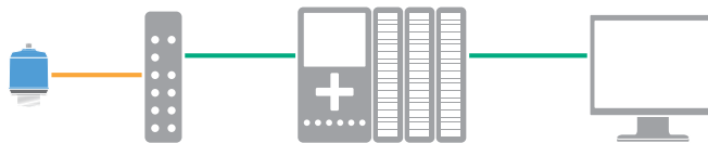
Figure 5-3: Connection via the PLC
