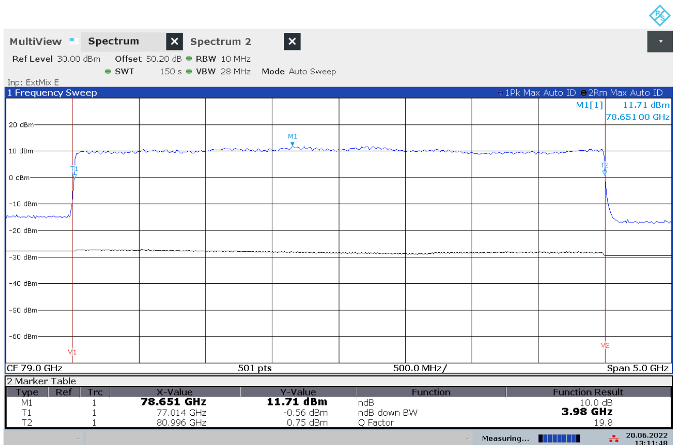
Plot 1: 10 dB bandwidth, Pos-Peak measurement, reference at 20°
