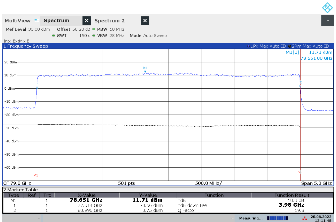
Plot 1: 10 dB bandwidth, Pos-Peak measurement, reference at 20°
