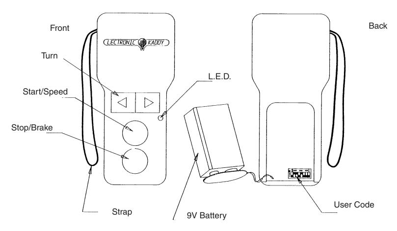
Replace Battery Open the transmitter case by sliding the battery cover to expose the battery. Remove the battery and disengage the polarized connector. Do not stress the wires by dangling the battery while still connected. Replace the battery with the specified alkaline battery. Replace the cover.
