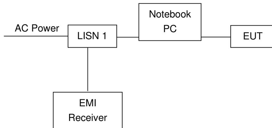
**Note:** The EUT was tested while in normal communication mode.
