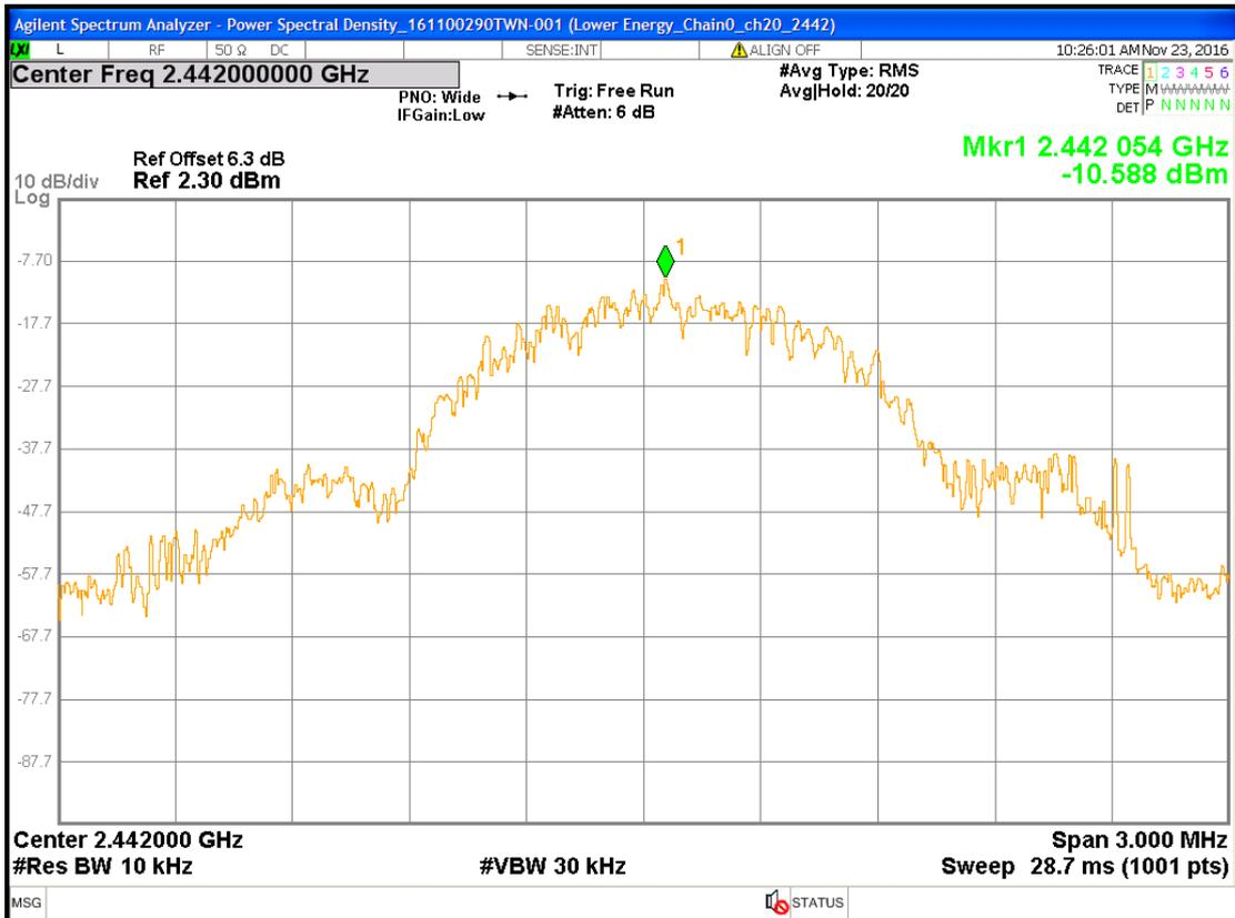
Chain0 : Power Spectral Density @ Lower Energy mode Ch high
