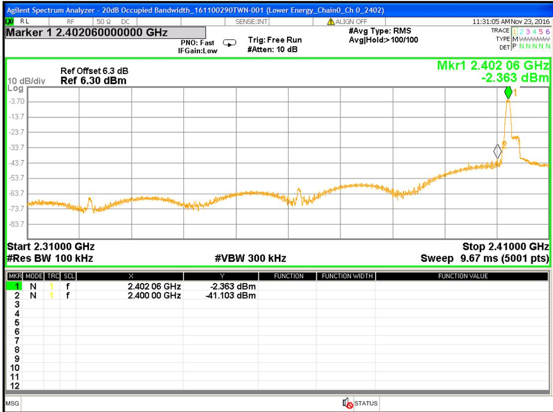
**Chain0 : Authorized-Band Band edge @ Lower Energy mode Ch high for RB8762-c-HM**
