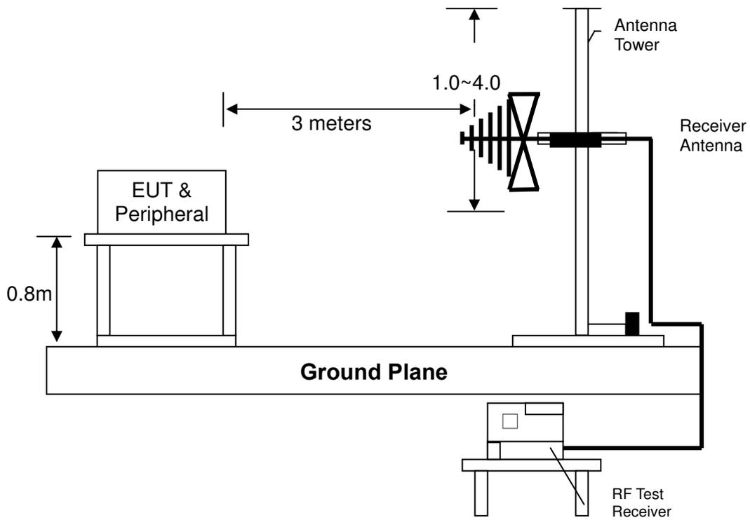
**7.5.3 Radiated emission above 1GHz using Horn Antenna**
