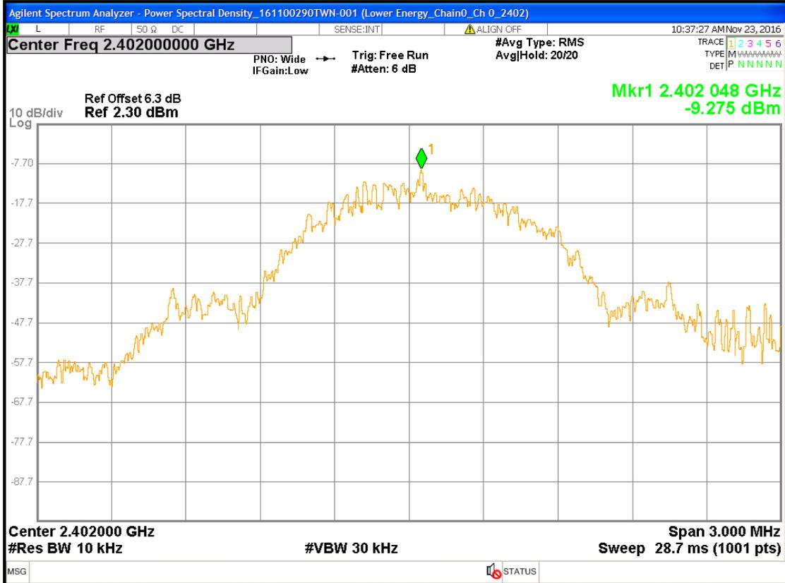
**Chain0 : Power Spectral Density @ Lower Energy mode Ch middle**
