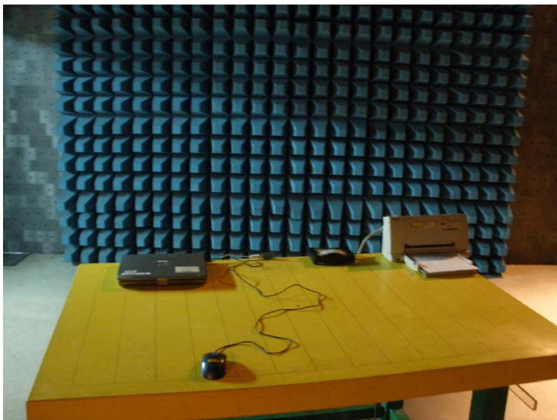
Photo 3: Radiated Emission Test set-up photo (WiFiHU-a-1-NE)
