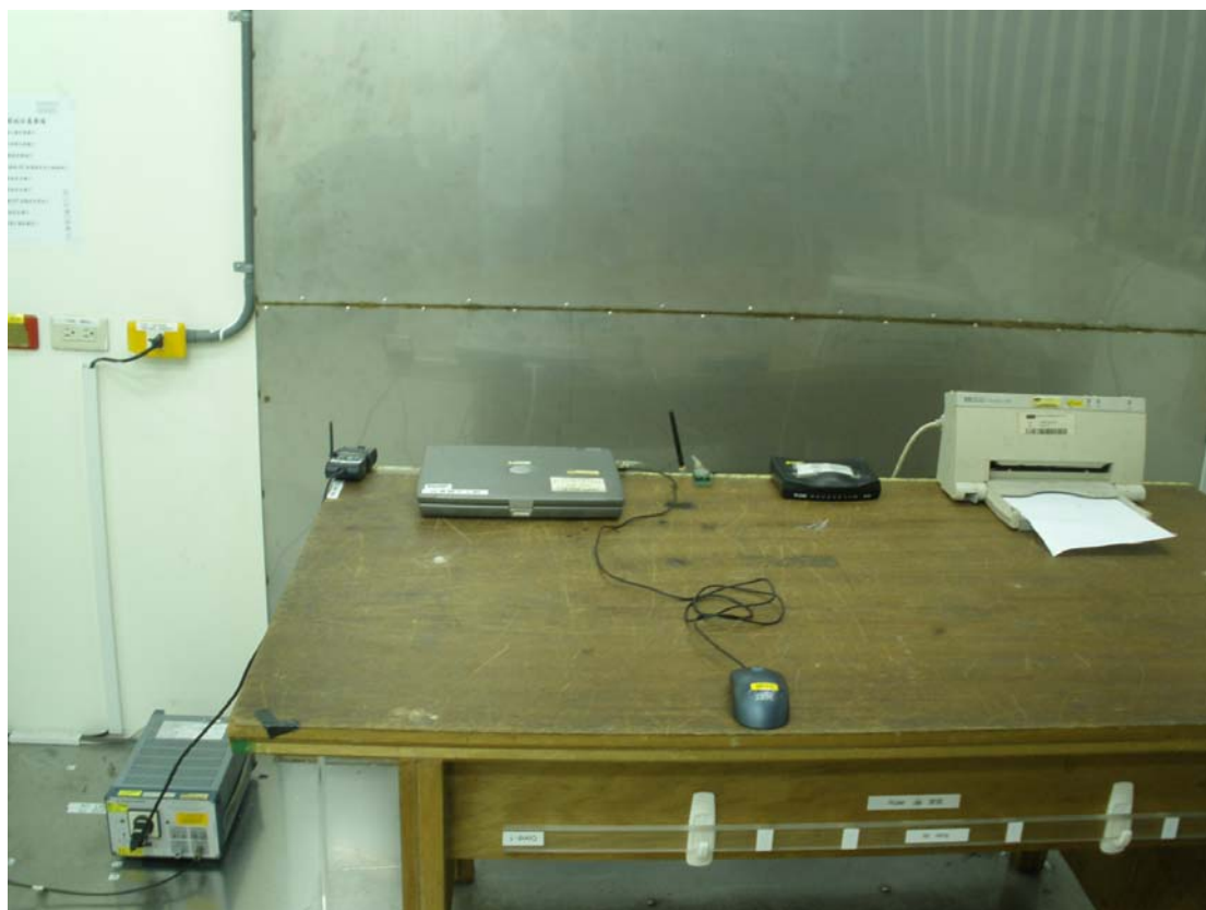
Photo 2: Conducted Emission Test Set-up photo (WiFiHU-c-1-NE)
