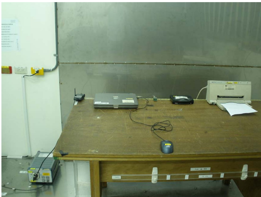
Photo 1: Conducted Emission Test Set-up photo (WiFiHU-a-1-NE)
