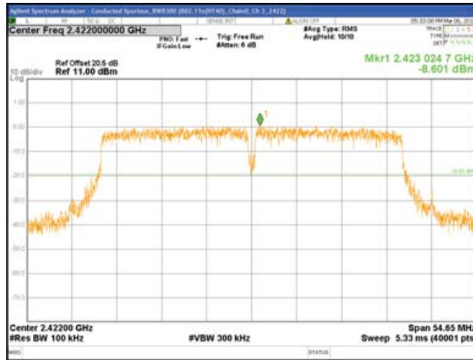
Chain0 : Conducted Spurious @ 802.11n(HT40) Mode Ch 3
