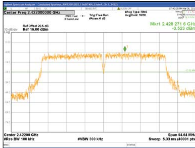
Chain1 : Conducted Spurious @ 802.11n(HT40) Mode Ch 3
