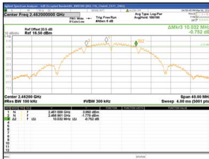
Chain0 : 6dB Bandwidth @ 802.11b Mode Ch11
