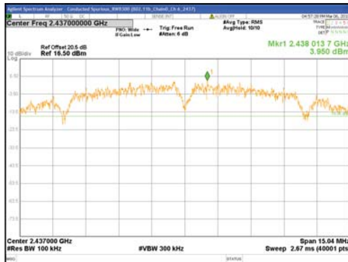
Chain0 : Conducted Spurious @ 802.11b Mode Ch 6
