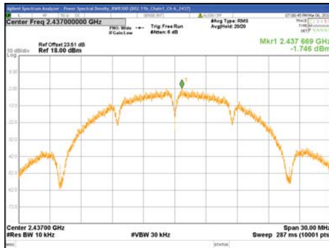
Chain1 : Power Spectral Density @ 802.11b Mode Ch11
