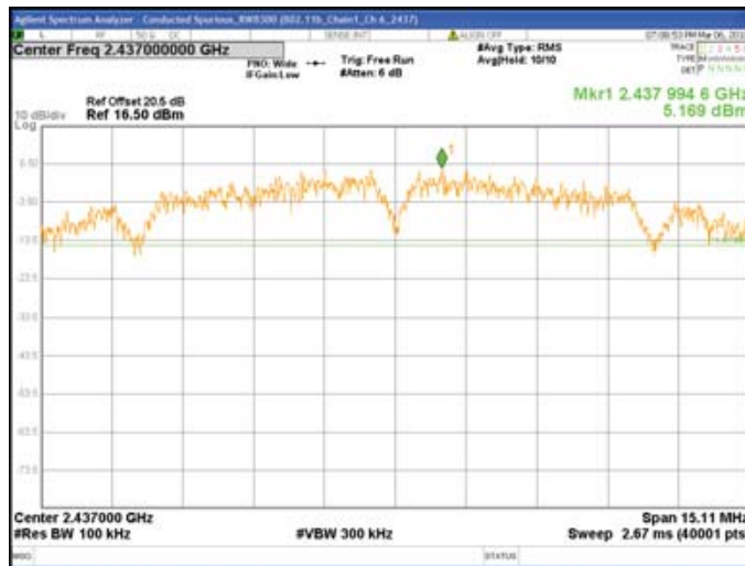
Chain1 : Conducted Spurious @ 802.11b Mode Ch 6
