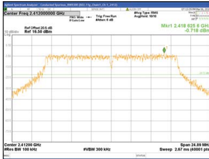
Chain1 : Conducted Spurious @ 802.11g Mode Ch 1
