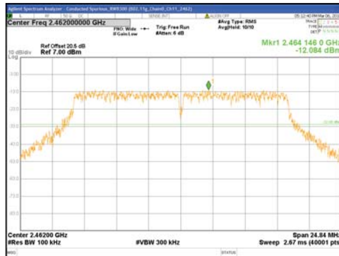
Chain0 : Conducted Spurious @ 802.11g Mode Ch11
