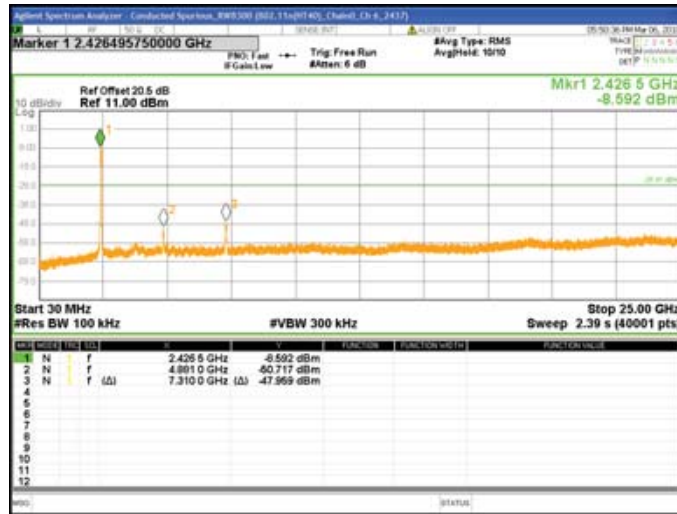
Chain0 : Conducted Spurious @ 802.11n(HT40) Mode Ch 9
