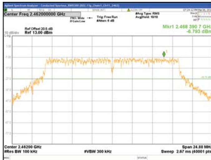
Chain1 : Conducted Spurious @ 802.11g Mode Ch11
