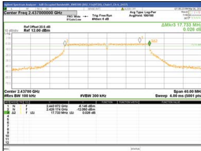
Chain1 : 6dB Bandwidth @ 802.11n(HT20) Mode Ch11
