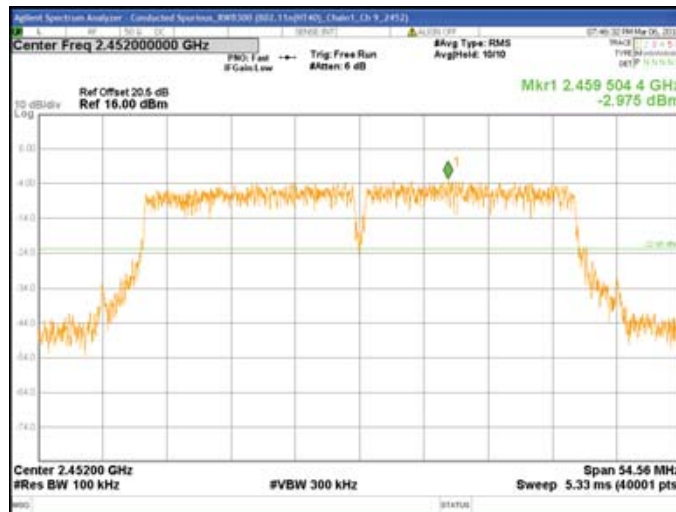
Chain1 : Conducted Spurious @ 802.11n(HT40) Mode Ch 9
