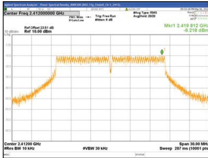
Chain0 : Power Spectral Density @ 802.11g Mode Ch 6
