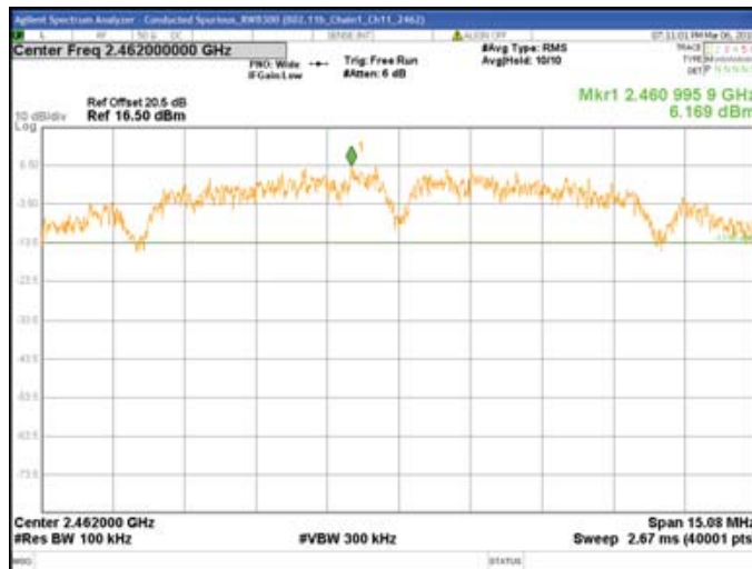
Chain1 : Conducted Spurious @ 802.11b Mode Ch11
