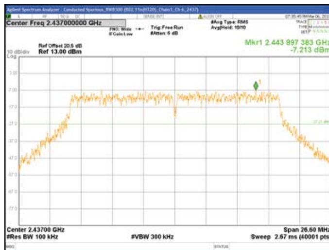
Chain1 : Conducted Spurious @ 802.11n(HT20) Mode Ch 6
