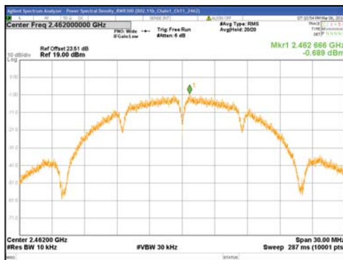
Chain1 : Power Spectral Density @ 802.11b Mode Ch11
