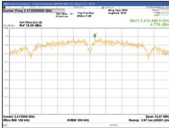
Chain1 : Conducted Spurious @ 802.11b Mode Ch 1
