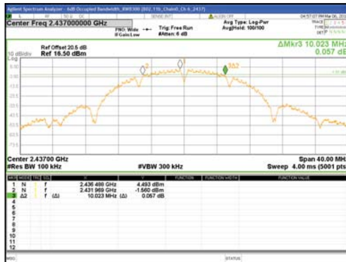
Chain0 : 6dB Bandwidth @ 802.11b Mode Ch11
