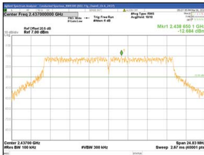
Chain0 : Conducted Spurious @ 802.11g Mode Ch 6
