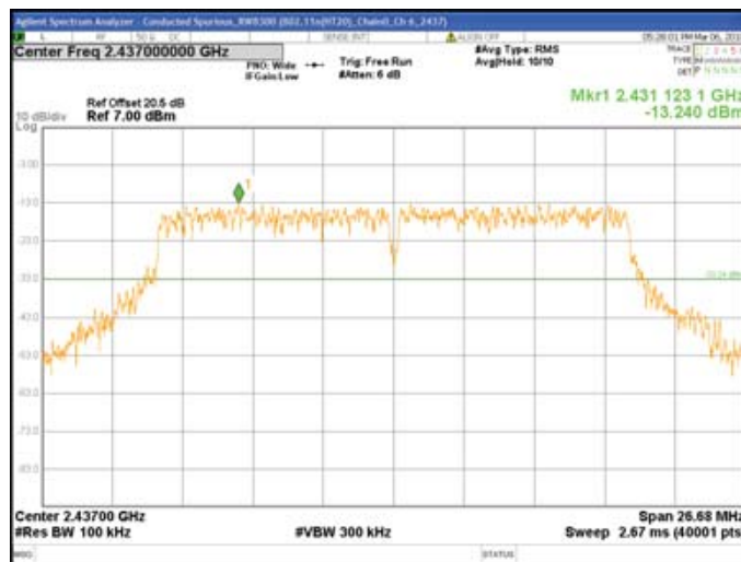
Chain0 : Conducted Spurious @ 802.11n(HT20) Mode Ch 6
