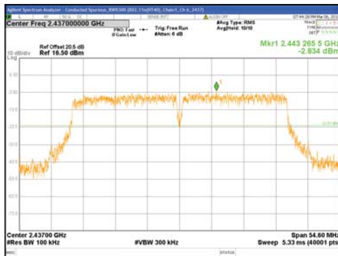
Chain1 : Conducted Spurious @ 802.11n(HT40) Mode Ch 6
