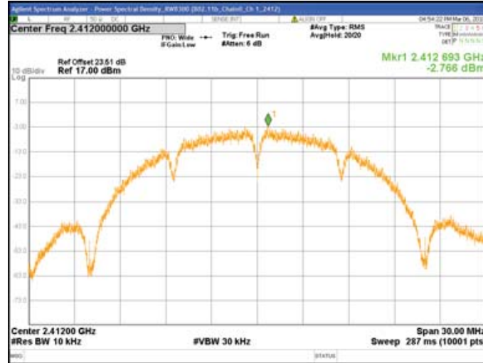
Chain0 : Power Spectral Density @ 802.11b Mode Ch 6
