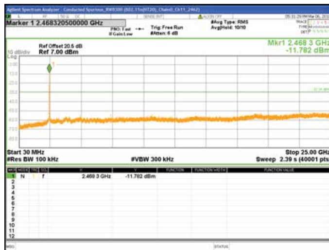
Chain0 : Conducted Spurious @ 802.11n(HT20) Mode Ch11
