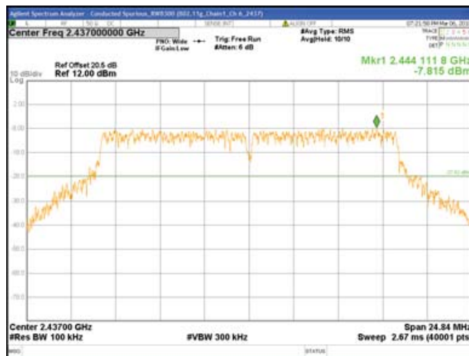
Chain1 : Conducted Spurious @ 802.11g Mode Ch 6
