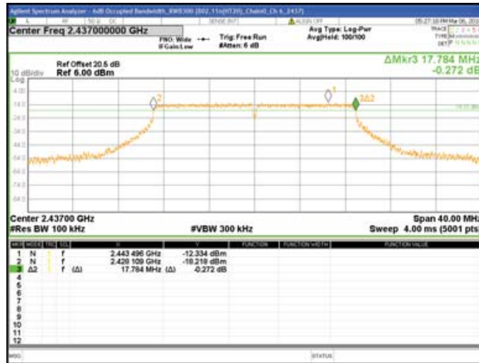
Chain0 : 6dB Bandwidth @ 802.11n(HT20) Mode Ch11
