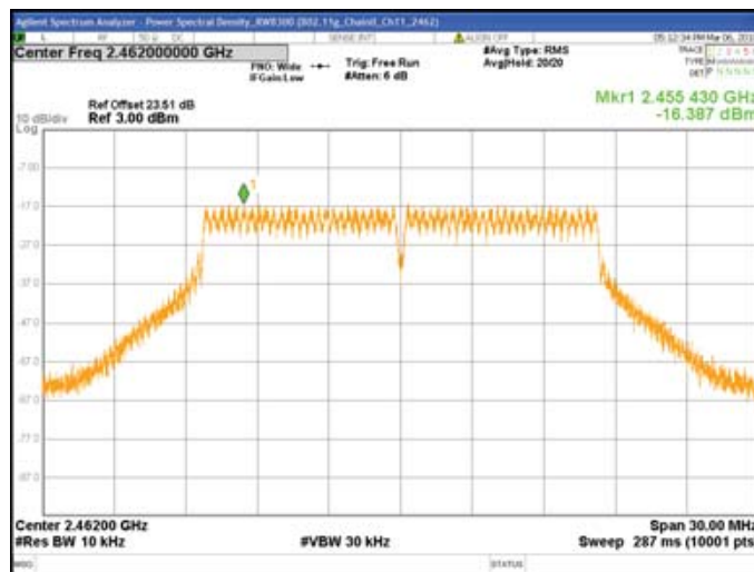
Chain0 : Power Spectral Density @ 802.11g Mode Ch11
