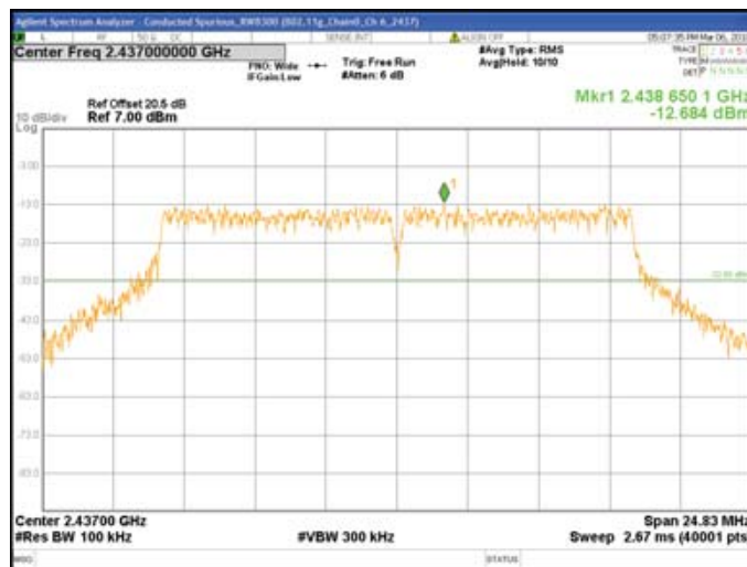
Chain0 : Conducted Spurious @ 802.11g Mode Ch 6
