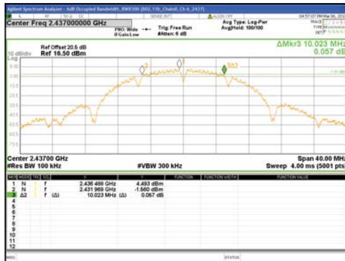
Chain0 : 6dB Bandwidth @ 802.11b Mode Ch11
