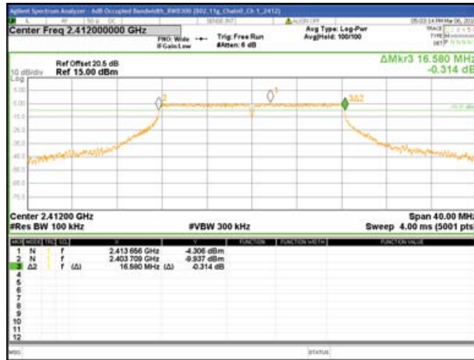
Chain0 : 6dB Bandwidth @ 802.11g Mode Ch 6
