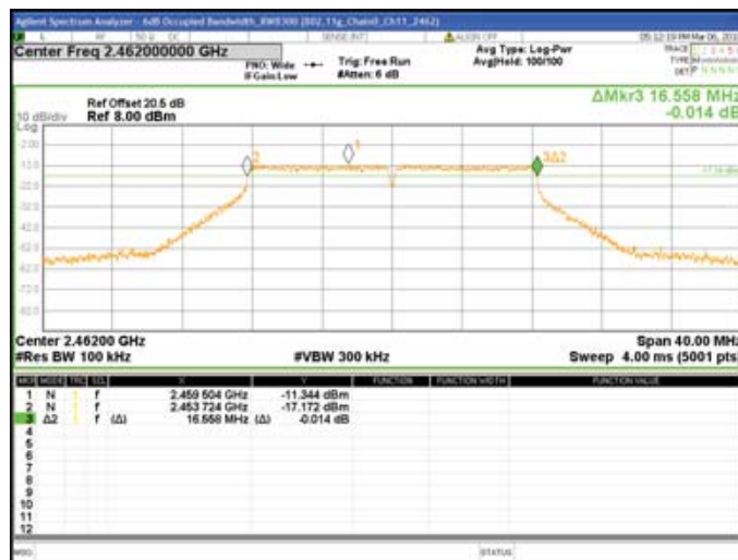
Chain0 : 6dB Bandwidth @ 802.11g Mode Ch11
