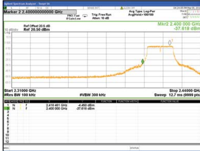
Chain1 : Authorized Band Bandedge @ 802.11n(HT20) Mode High
