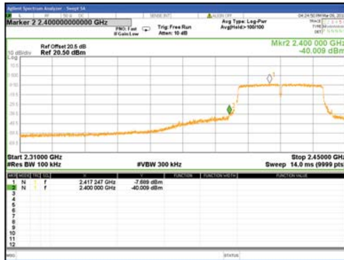
Chain1 : Authorized Band Bandedge @ 802.11n(HT40) Mode High
