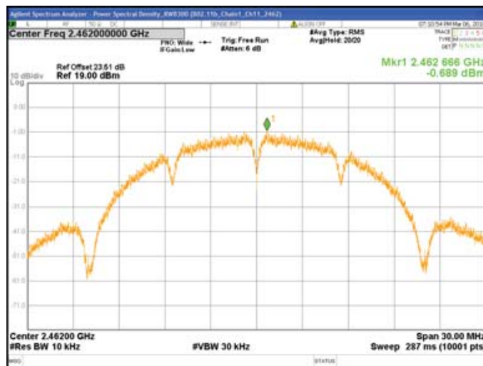
Chain1 : Power Spectral Density @ 802.11b Mode Ch11
