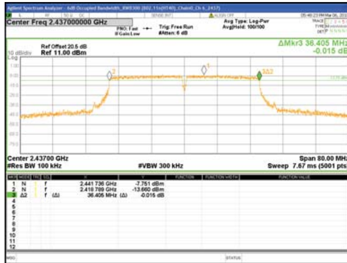
Chain0 : 6dB Bandwidth @ 802.11n(HT40) Mode Ch 9
