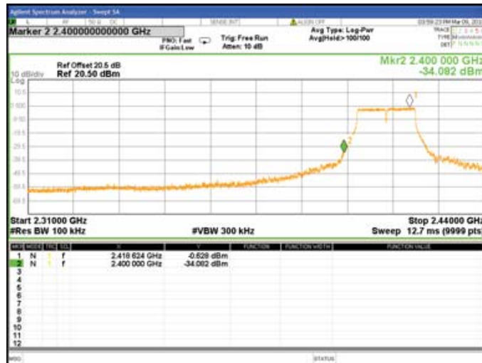
Chain0 : Authorized Band Bandedge @ 802.11n(HT20) Mode High
