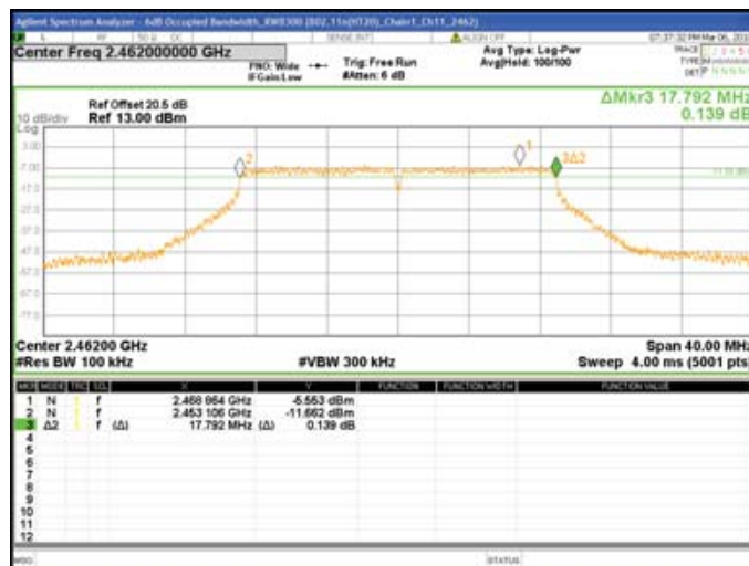
Chain1 : 6dB Bandwidth @ 802.11n(HT20) Mode Ch11
