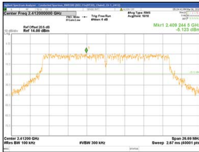
Chain0 : Conducted Spurious @ 802.11n(HT20) Mode Ch 1
