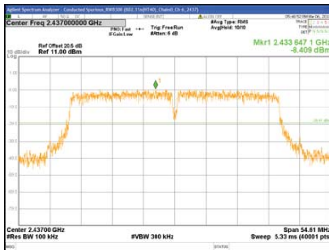
Chain0 : Conducted Spurious @ 802.11n(HT40) Mode Ch 6
