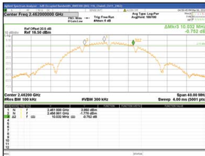
Chain0 : 6dB Bandwidth @ 802.11b Mode Ch11
