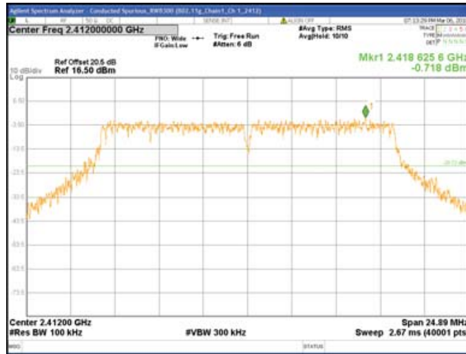
Chain1 : Conducted Spurious @ 802.11g Mode Ch 1
