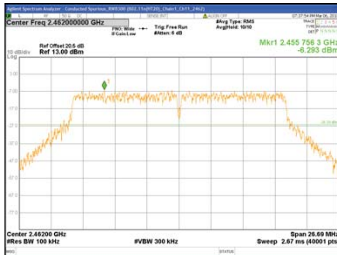
Chain1 : Conducted Spurious @ 802.11n(HT20) Mode Ch11
