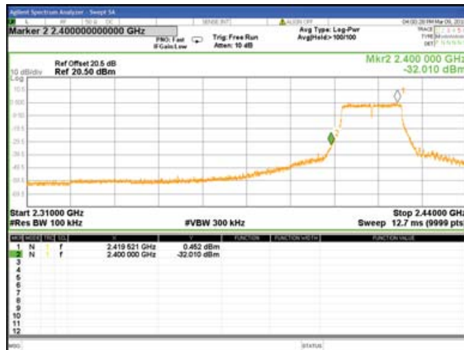
Chain1 : Authorized Band Bandedge @ 802.11n(HT20) Mode Low
