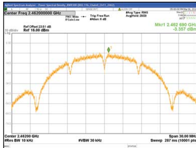
Chain0 : Power Spectral Density @ 802.11b Mode Ch11
