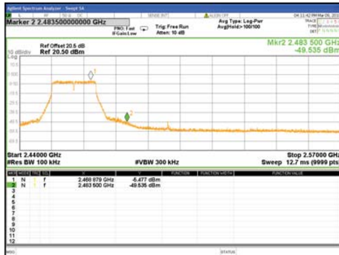
Chain1 : Authorized Band Bandedge @ 802.11n(HT20) Mode Low
