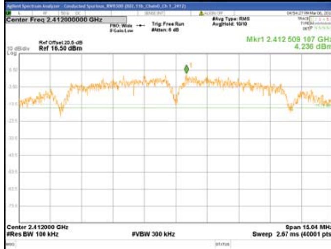
Chain0 : Conducted Spurious @ 802.11b Mode Ch 1
