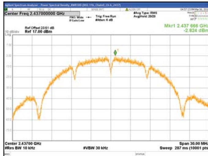
Chain0 : Power Spectral Density @ 802.11b Mode Ch11
