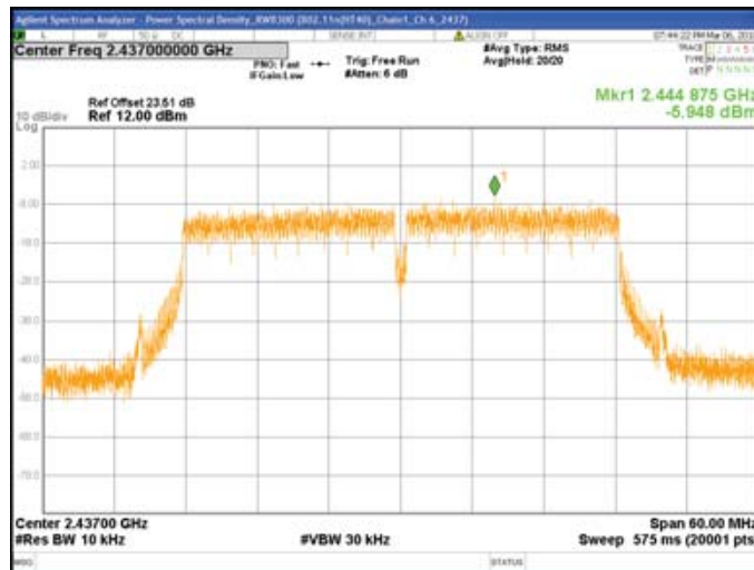
Chain1 : Power Spectral Density @ 802.11n(HT40) Mode Ch 9
