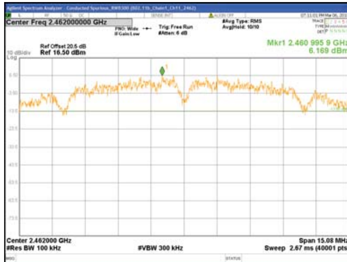
Chain1 : Conducted Spurious @ 802.11b Mode Ch11
