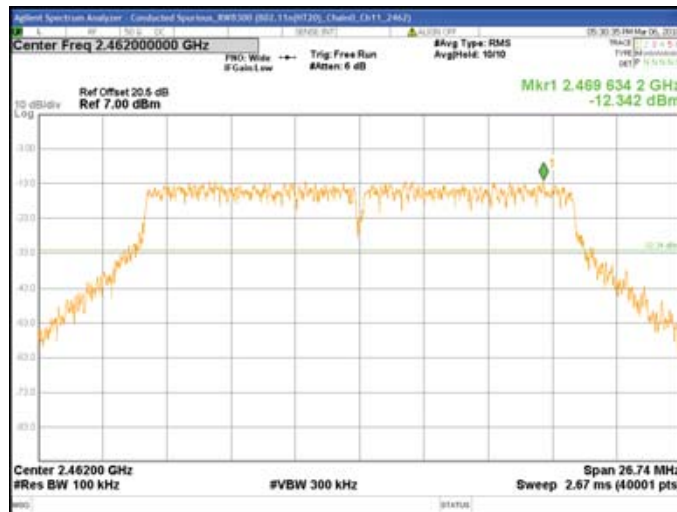
Chain0 : Conducted Spurious @ 802.11n(HT20) Mode Ch11
