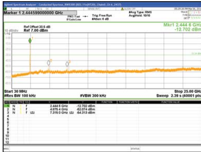
Chain0 : Conducted Spurious @ 802.11n(HT20) Mode Ch11
