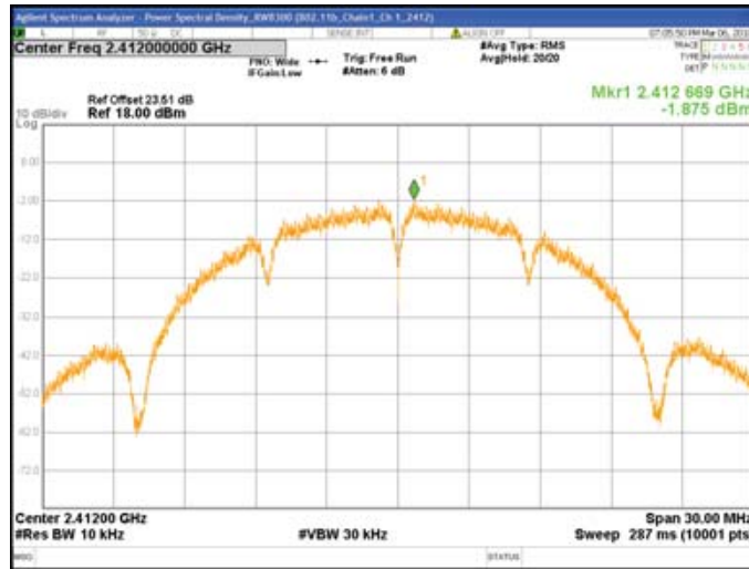
Chain1 : Power Spectral Density @ 802.11b Mode Ch 6
