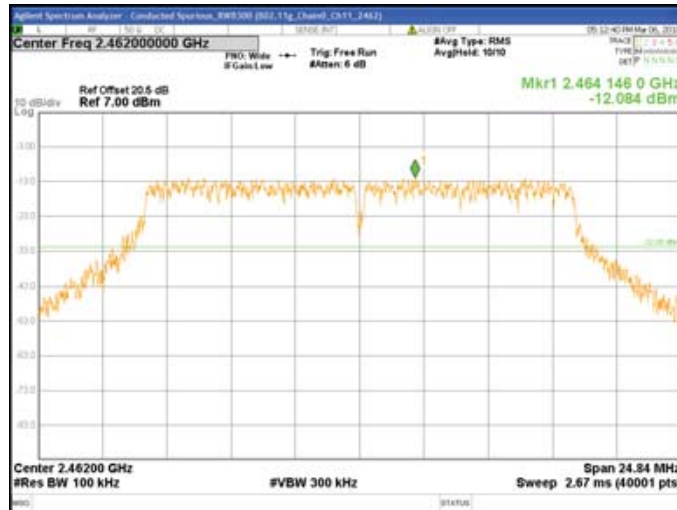
Chain0 : Conducted Spurious @ 802.11g Mode Ch11
