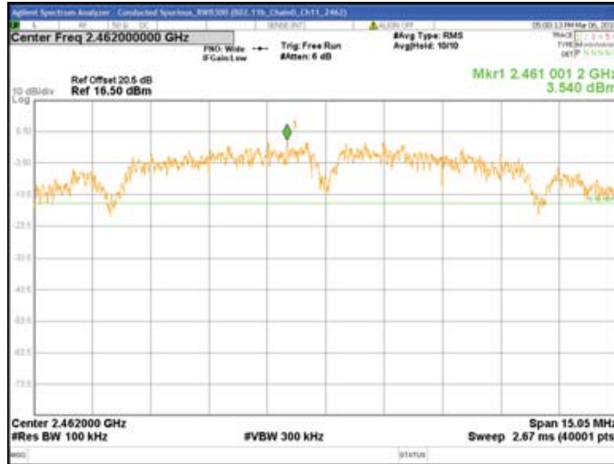
Chain0 : Conducted Spurious @ 802.11b Mode Ch11
