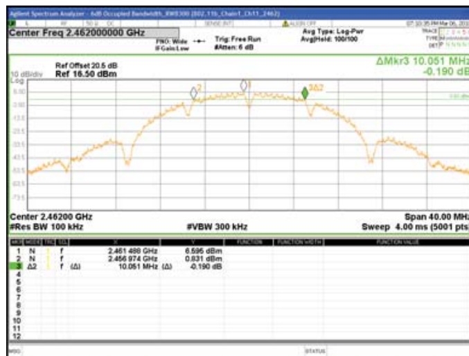
Chain1 : 6dB Bandwidth @ 802.11b Mode Ch11
