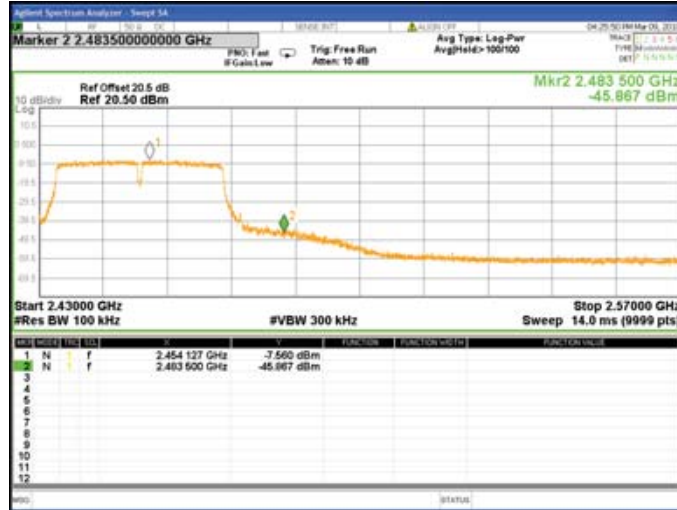
Chain0 : Authorized Band Bandedge @ 802.11n(HT40) Mode Low
