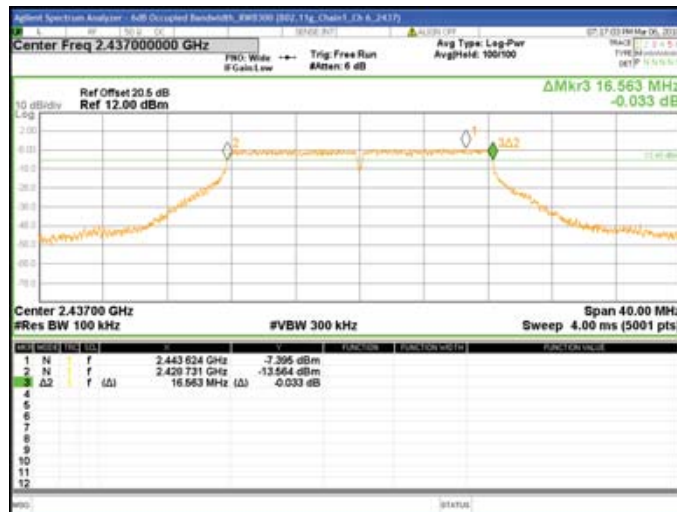
Chain1 : 6dB Bandwidth @ 802.11g Mode Ch11
