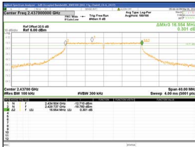
Chain0 : 6dB Bandwidth @ 802.11g Mode Ch11
