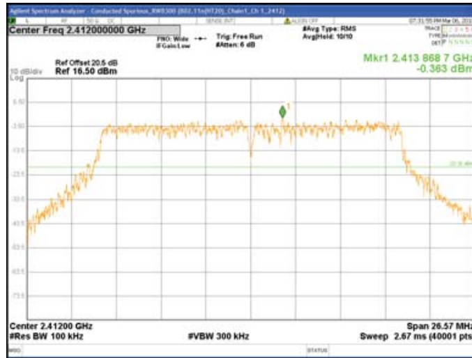
Chain1 : Conducted Spurious @ 802.11n(HT20) Mode Ch 1
