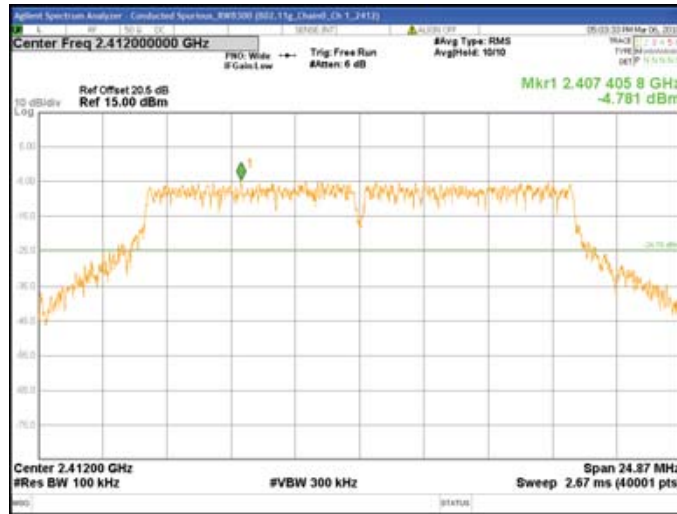
Chain0 : Conducted Spurious @ 802.11g Mode Ch 1
