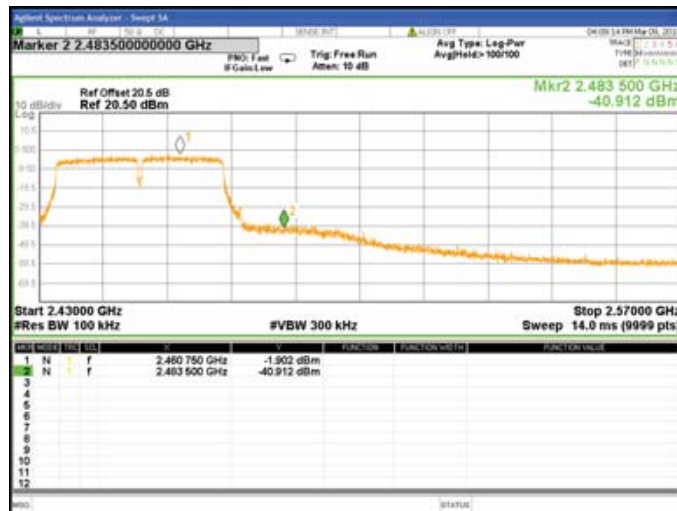
Chain1 : Authorized Band Bandedge @ 802.11n(HT40) Mode High
