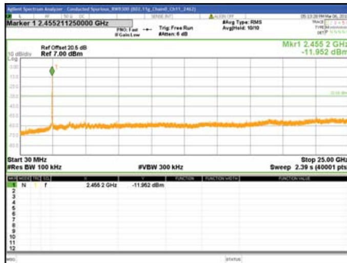
Chain0 : Conducted Spurious @ 802.11g Mode Ch11
