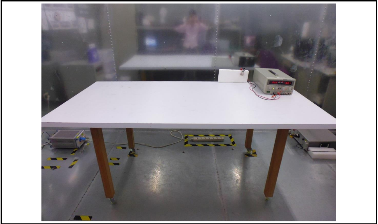
Conducted Emission Test (for model RB540-a)
