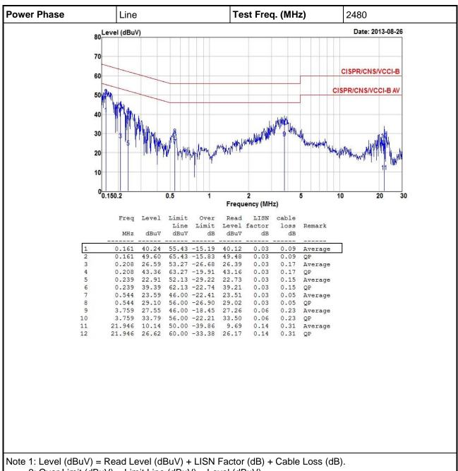
2: Over Limit (dBuV) = Limit Line (dBuV) - Level (dBuV).
