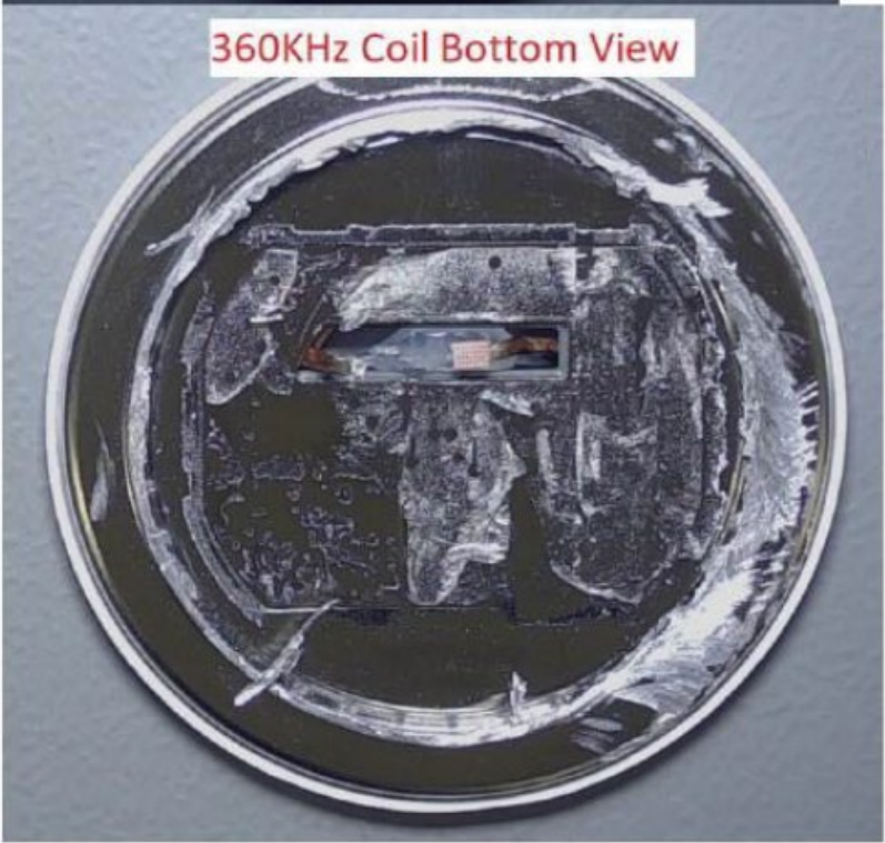
C222x Coil Antenna (MagSafe iPhones – 360 kHz) – Bottom View
