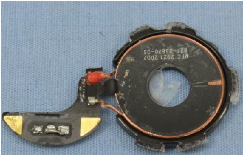
C962 PCB (Apple Watch – 326.5kHz/1.778MHz) – Bottom View
