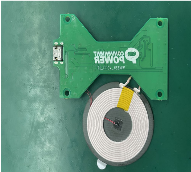
PCB with A11a AirPods PCB (AirPods – 110.5kHz to 148kHz) – Bottom View
