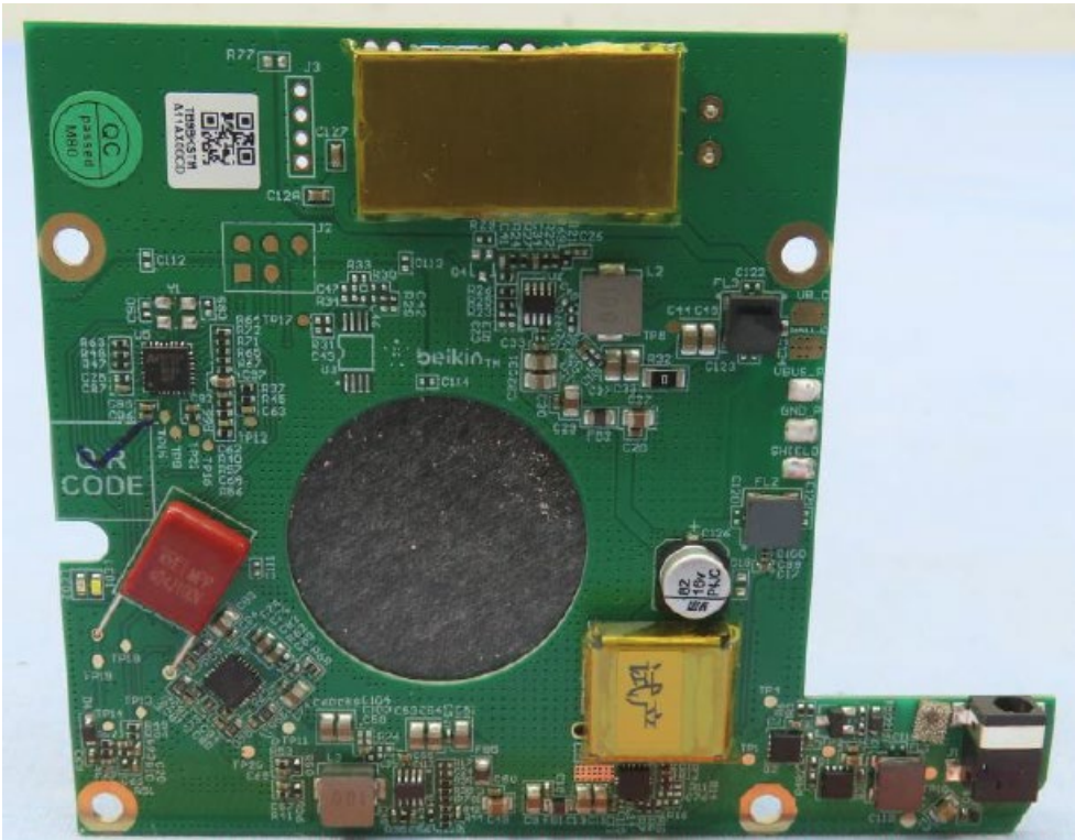
Center Coil Antenna for AirPods (110.5 kHz to 148.5 kHz) – Bottom View
