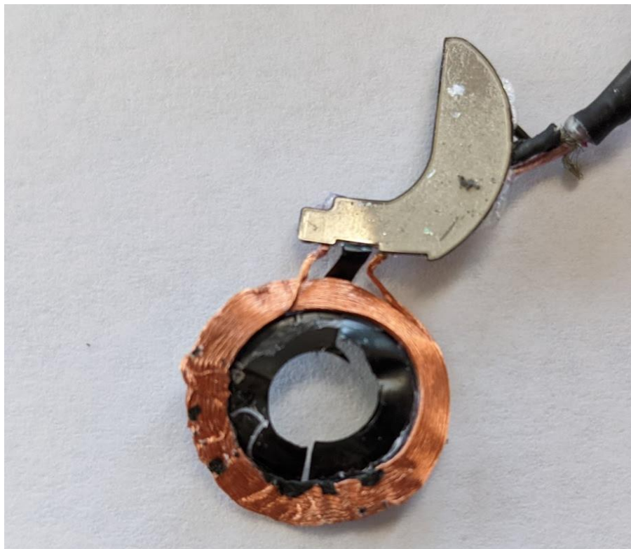
326.5kHz + 1.778 MHz Apple Watch Coil (Bottom)
