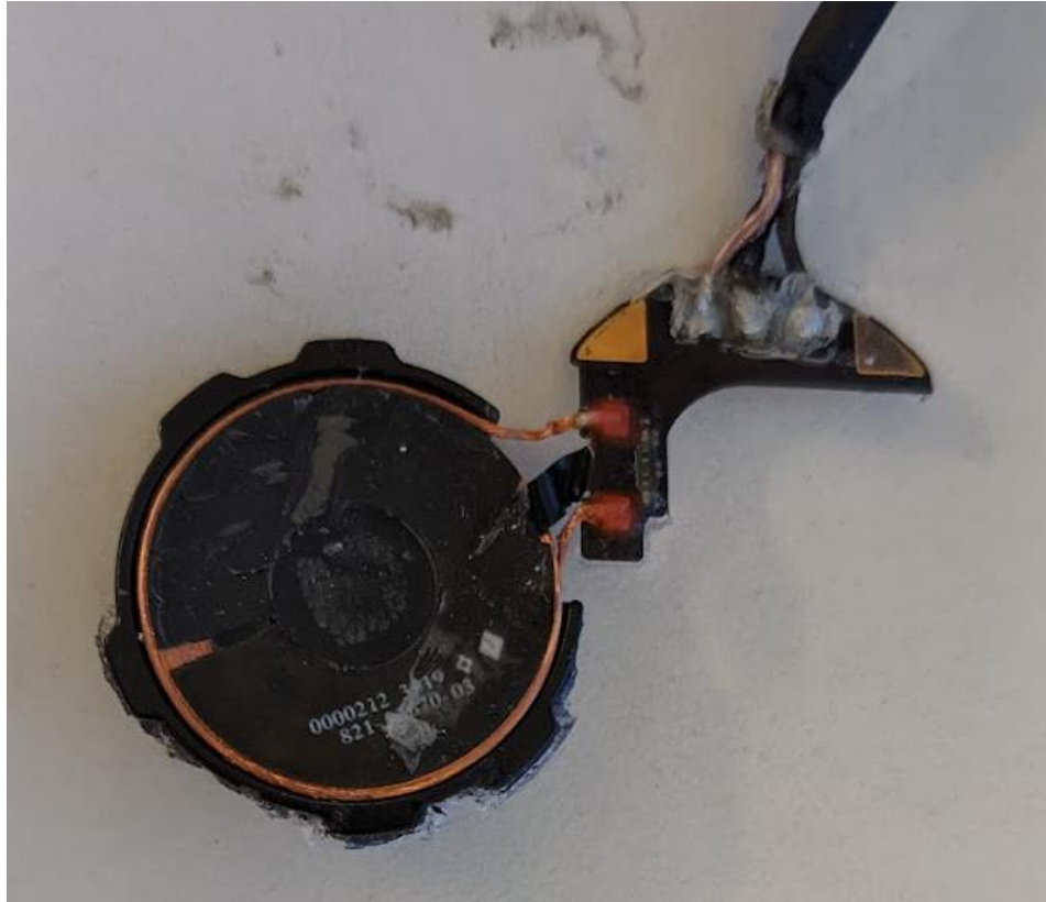
326.5kHz + 1.778 MHz Apple Watch Coil (Bottom)
