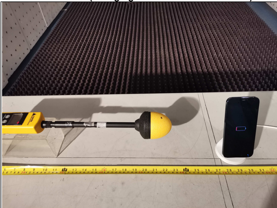
Electric Field (Charging mode with iPhone 12 Pro)
