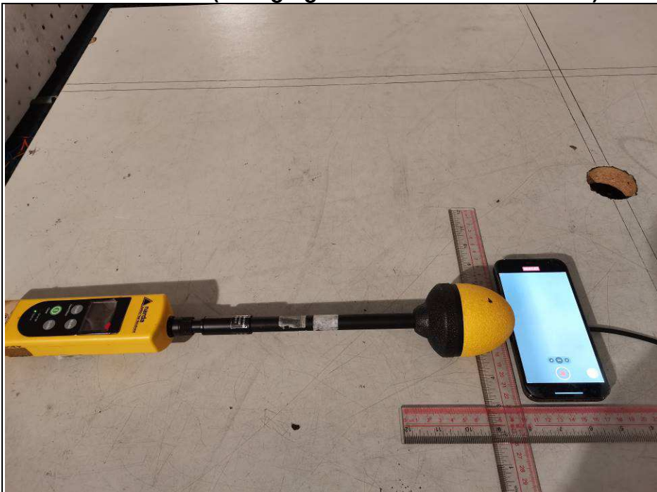
Electric Field (Charging mode with iPhone 12 Pro)
