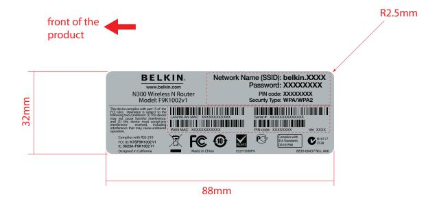
Elements within red boxes are to be printed in BLACK on pre-printed label at the factory.
