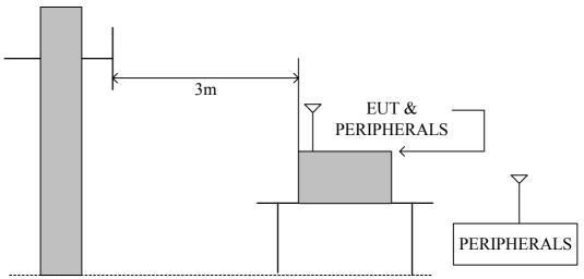
Antenna Elevation Variable
