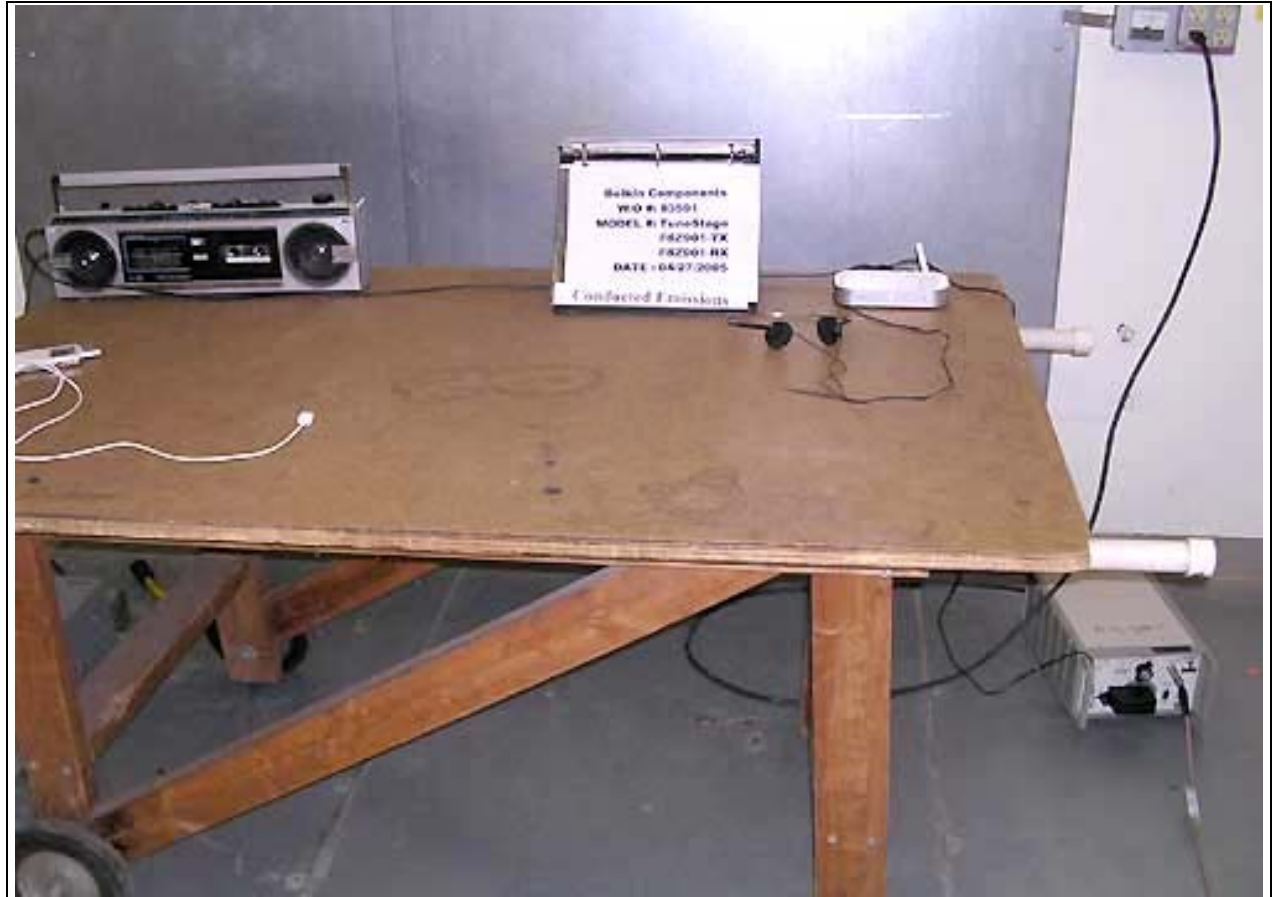
Mains Conducted Emissions - Front View - F8Z901-RX
