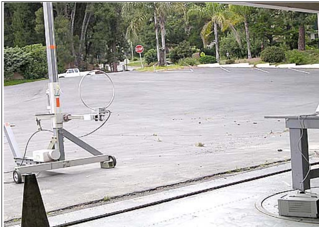
Radiated Emissions - Front View - Loop Antenna
