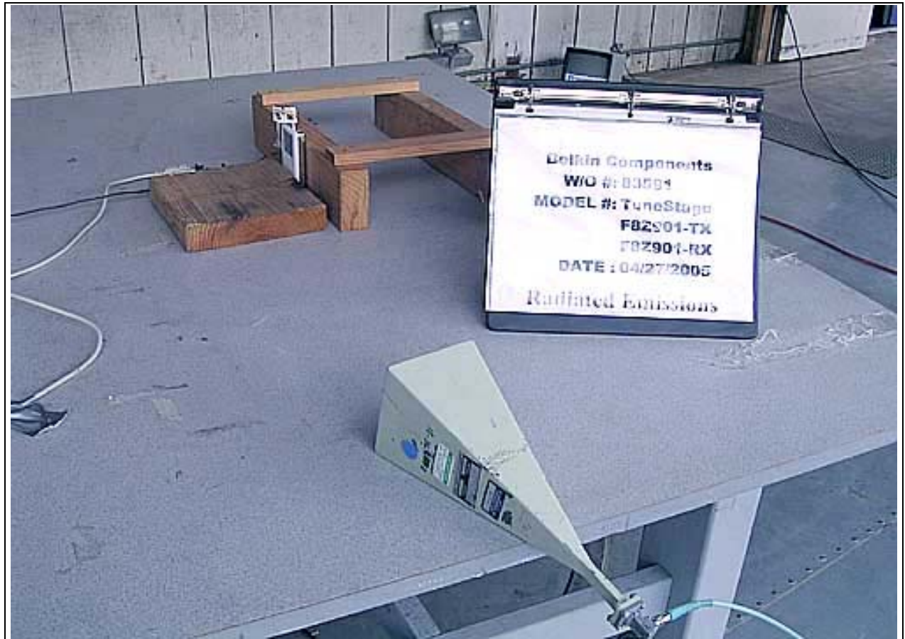
Radiated Emissions - Front View - Horn Antenna
