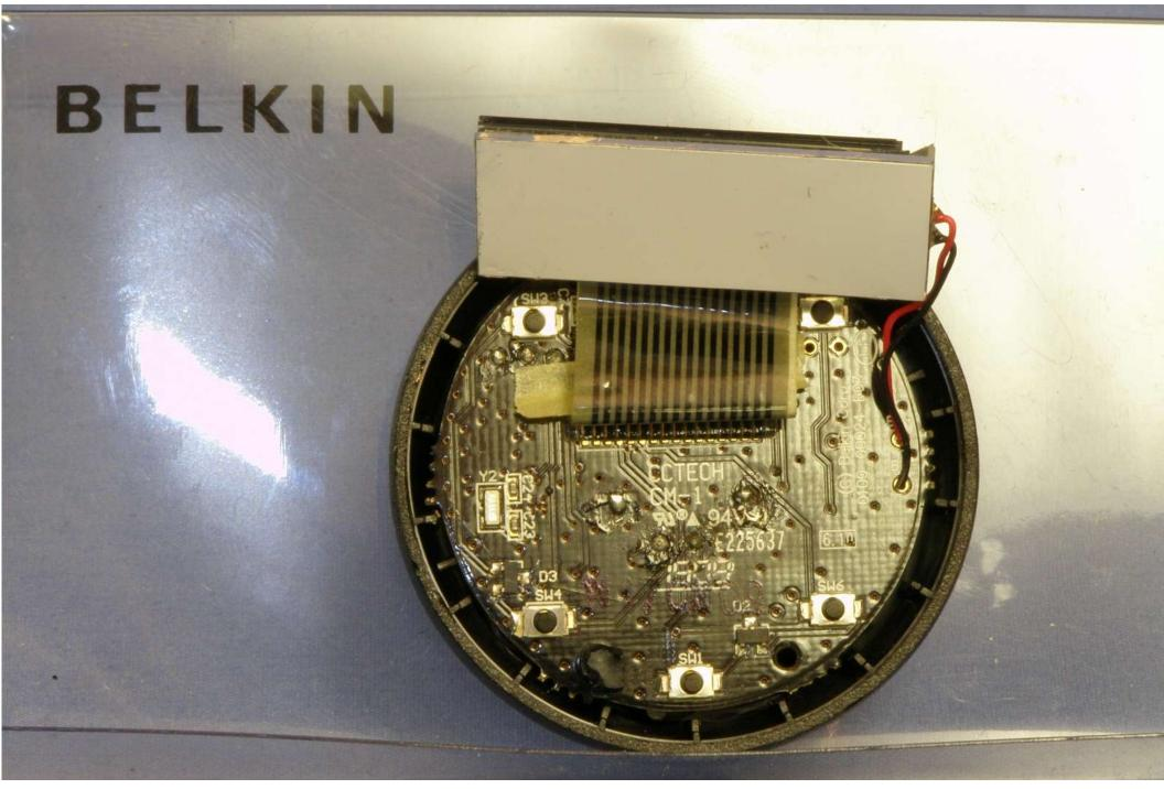
Photo 12 - Top side of Processor Board
