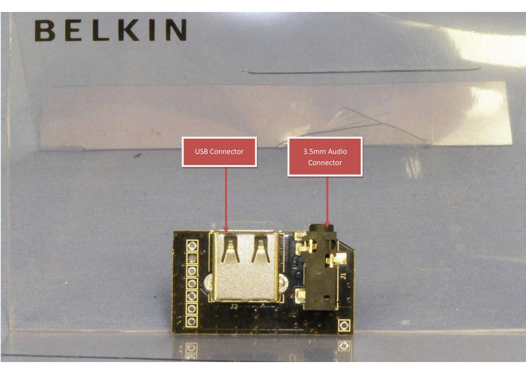
Photo 8 - Bottom Side of Connector Board
