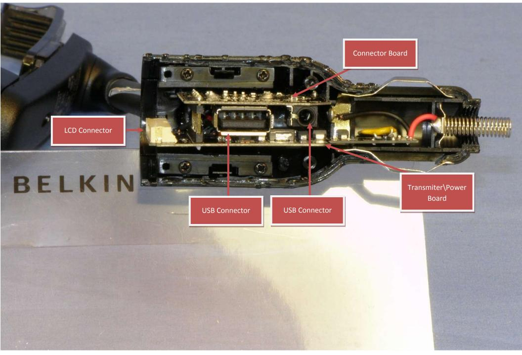
Photo 6 - Side of Transmitter\ Power\Connector Board
