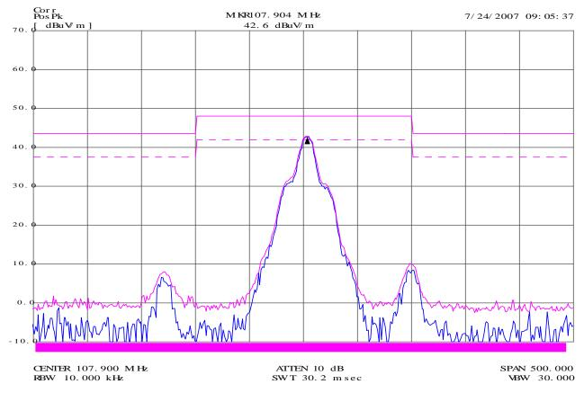
Figure 6 - Channel 107.9MHz Band edge Results for Vertical
