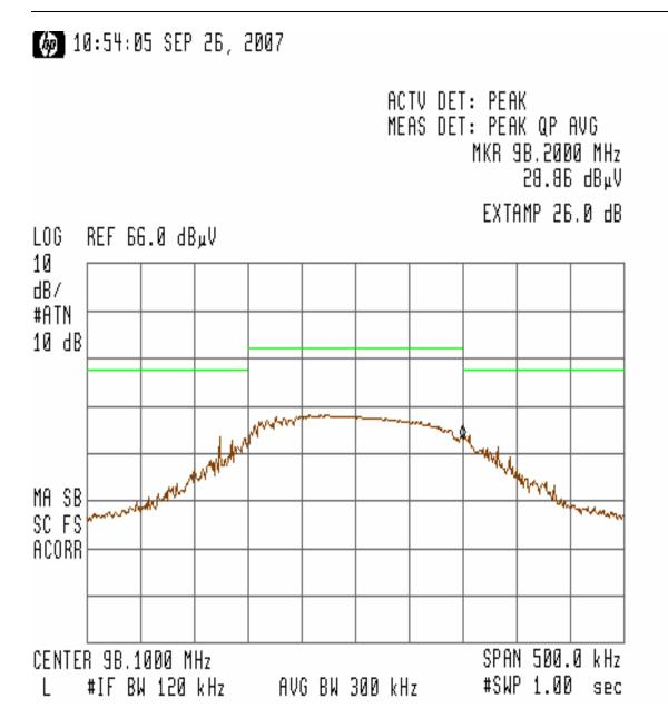
Figure 18 – Bandedge Measurement for Channel 98.1MHz (Horizontal) at 15.87VDC
