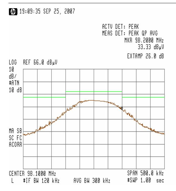
Figure 19 – Bandedge Measurement for Channel 98.1MHz (Vertical) at 11.73VDC
