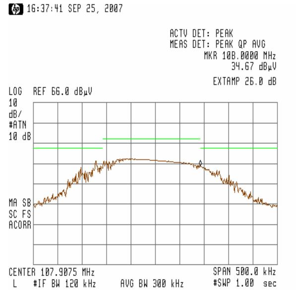
Figure 22 - Bandedge Measurement for Channel 107.9MHz (Horizontal) at 15.87VDC
