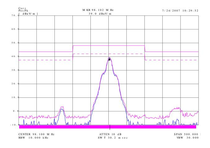
Figure 4 – Channel 98.1MHz Band edge Results for Vertical
