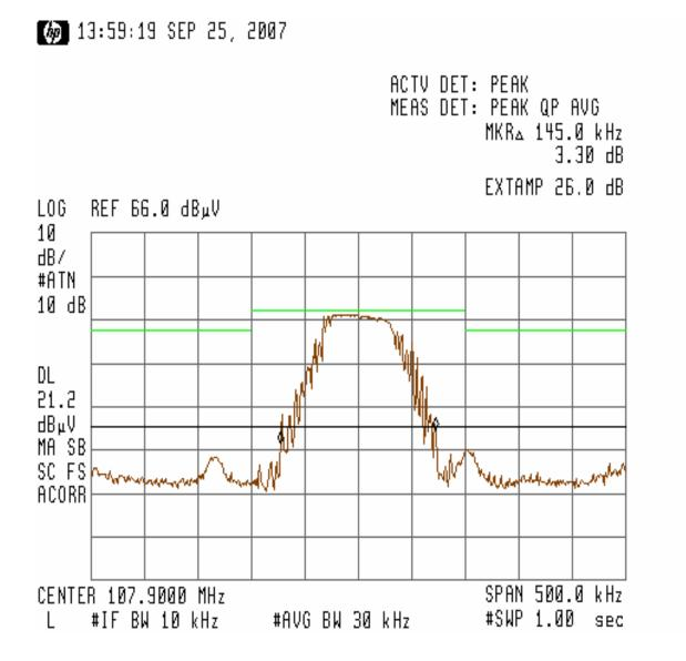
Figure 12 – Channel 107.9MHz (Vertical) – 26dB Bandwidth with 200 kHz Bandwidth Envelope Note: The TBFM2 was positioned on its side.
