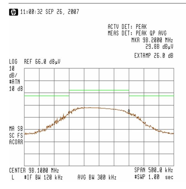
Figure 17 – Bandedge Measurement for Channel 98.1MHz (Horizontal) at 11.73VDC Note: The TBFM2 was positioned on the Side position.
