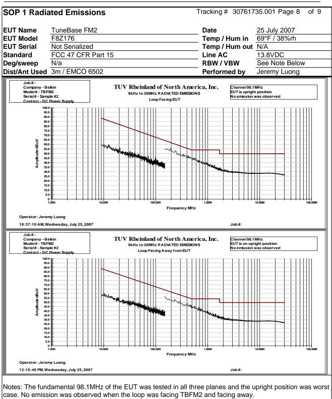
Receiver Setting: 9kHz-150kHz Range - IFW (200Hz) / VBW (300Hz) 150kHz-30MHz Range – IFBW (10kHz) / VBW (30kHz)
