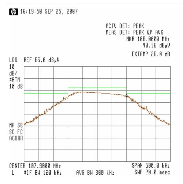
Figure 24 – Bandedge Measurement for Channel 107.9MHz (Vertical) at 15.87VDC
