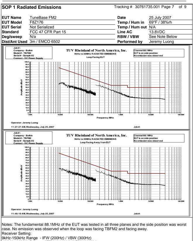
150kHz-30MHz Range – IFBW (10kHz) / VBW (30kHz)
