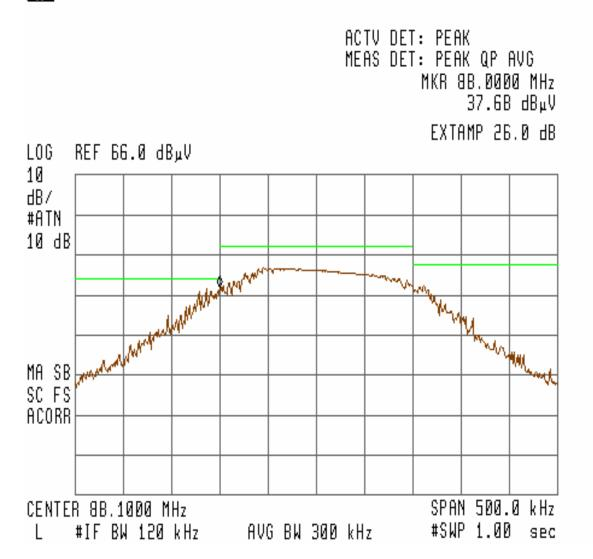
Figure 15 – Bandedge Measurement for Channel 88.1MHz (Vertical) at 11.73VDC
