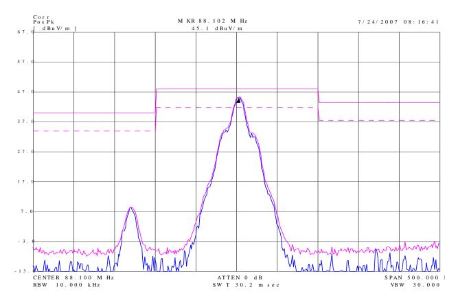
Figure 1 – Channel 88.1 Band edge Results for Horizontal
