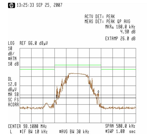
Figure 9 – Channel 98.1MHz (Horizontal) – 26dB Bandwidth with 200 kHz Bandwidth Envelope Note: The TBFM2 was positioned on its side.
