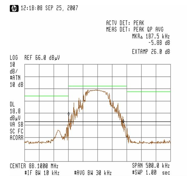
Figure 8 - Channel 88.1MHz (Vertical) - 26dB Bandwidth with 200 kHz Bandwidth Envelope
