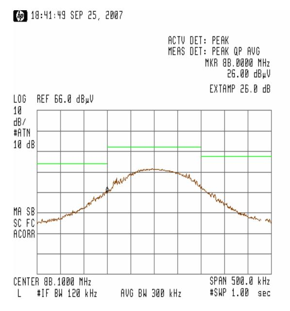
Figure 13 - Bandedge Measurement for Channel 88.1MHz (Horizontal) at 11.73VDC
