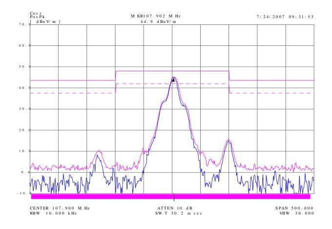
Figure 5 – Channel 107.9MHz Band edge Results for Horizontal
