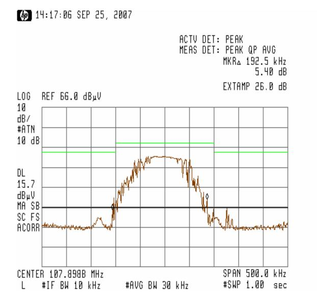
Figure 11 – Channel 107.9MHz (Horizontal) – 26dB Bandwidth with 200 kHz Bandwidth Envelope Note: The TBFM2 was positioned on its side.
