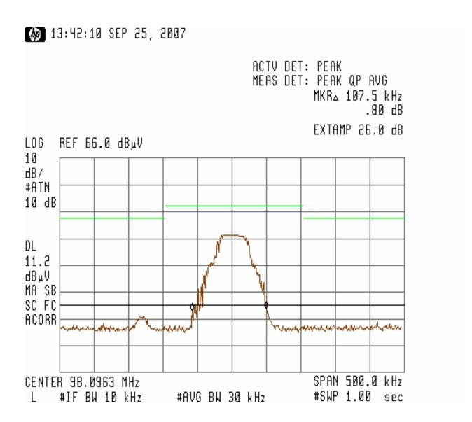
Figure 10 – Channel 98.1MHz (Vertical) – 26dB Bandwidth with 200 kHz Bandwidth Envelope Note: The TBFM2 was positioned on its upright.
