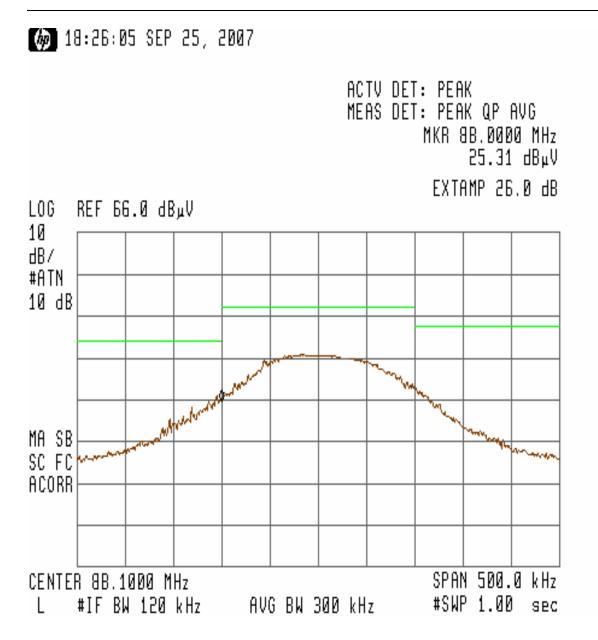
Figure 14 – Bandedge Measurement for Channel 88.1MHz (Horizontal) at 15.87VDC Note: The TBFM2 was positioned on the Side position.
