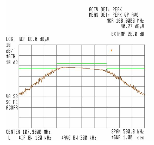
Figure 23 – Bandedge Measurement for Channel 107.9MHz (Vertical) at 11.73VDC
