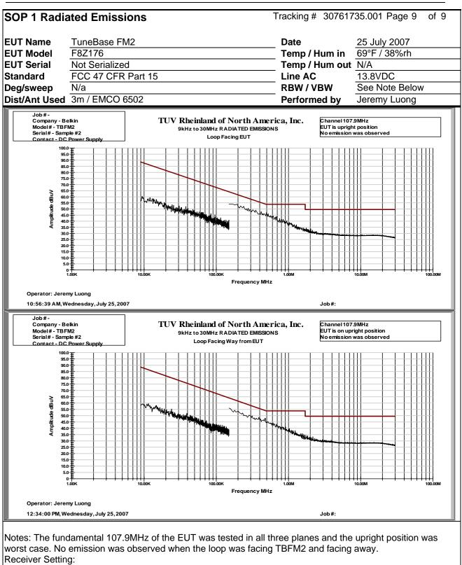
9kHz-150kHz Range - IFW (200Hz) / VBW (300Hz) 150kHz-30MHz Range – IFBW (10kHz) / VBW (30kHz)
