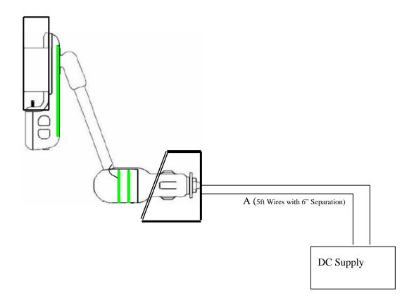
Figure 25 - Block Diagram of EUT Set-Up
