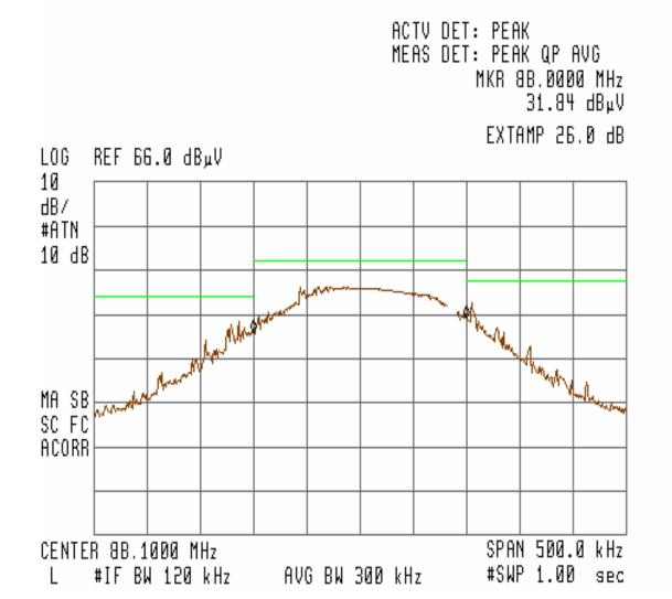
Figure 16 – Bandedge Measurement for Channel 88.1MHz (Vertical) at 15.87VDC
