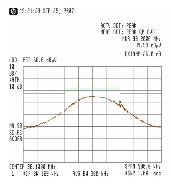
Figure 20 – Bandedge Measurement for Channel 98.1MHz (Vertical) at 15.87VDC
