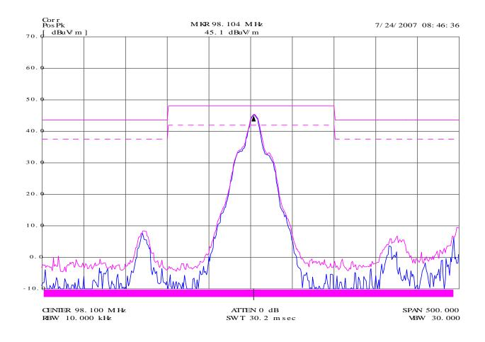
Figure 3 – Channel 98.1MHz Band edge Results for Horizontal
