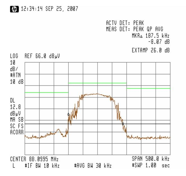
Figure 7 – Channel 88.1MHz (Horizontal), 26dB Bandwidth with 200 kHz Bandwidth Envelope
