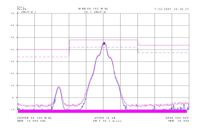
Figure 2 - Channel 88.1MHz Band edge Results for Vertical
