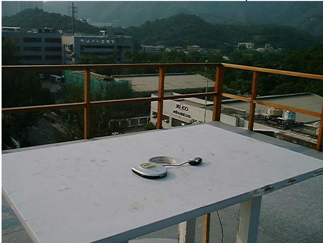
Measurement of Radiated Emission Test Set Up
