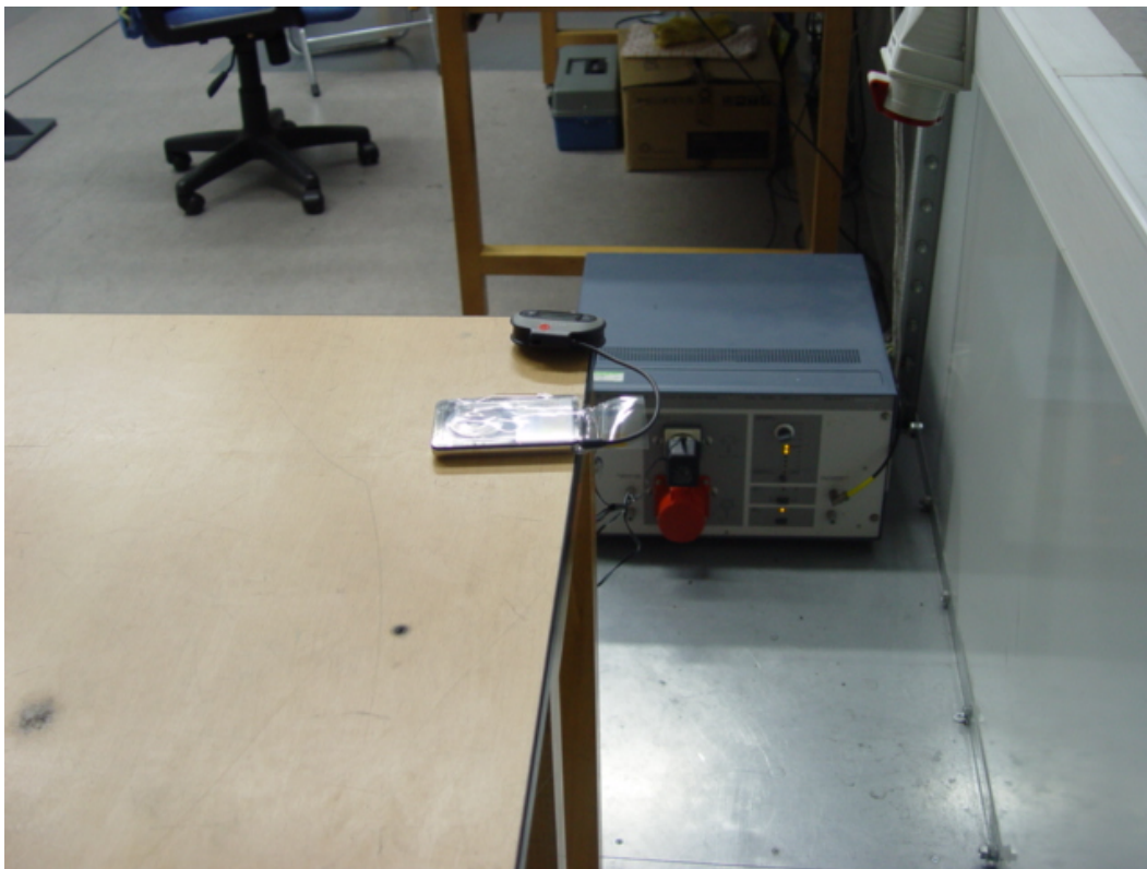
Photo 2 Conducted Emission Test
