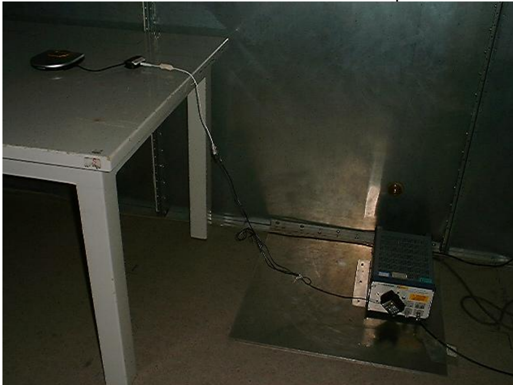
Measurement of Conducted Emission Test Set Up
