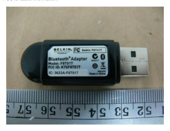
The label size is 22.7 mm X 11.9 mm and because of the size of this device is too small to be placed the other required statement, the following will be placed in the user's manual:
