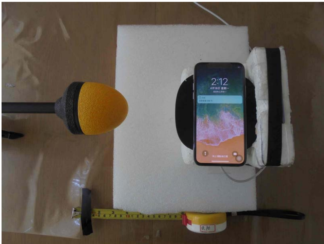
E-Field (Charging Mode with iPhone X - Z-axis)
