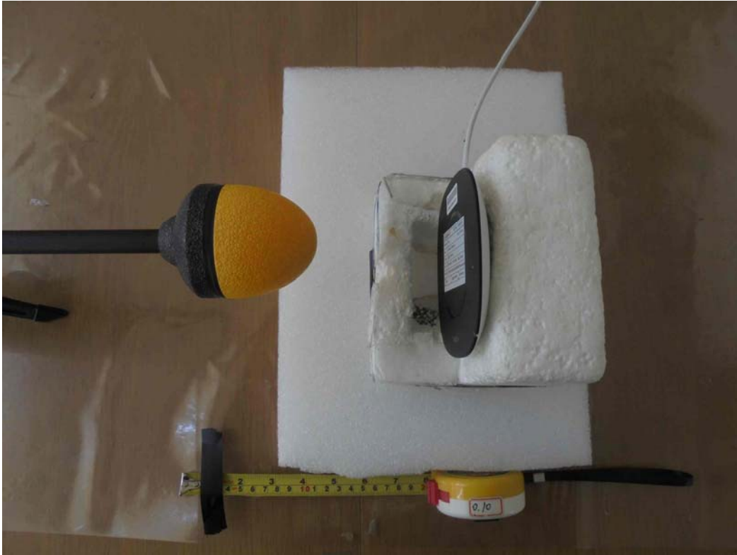
H-Field (Charging Mode with Load - Top)
