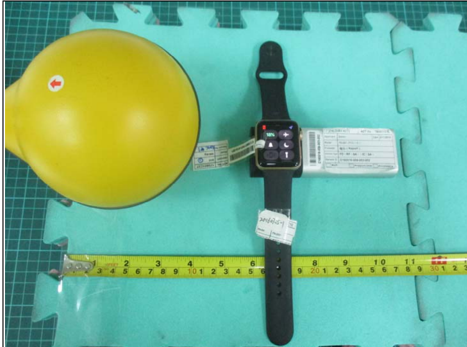
H-Field (Bottom) (Charging Mode) 15cm
