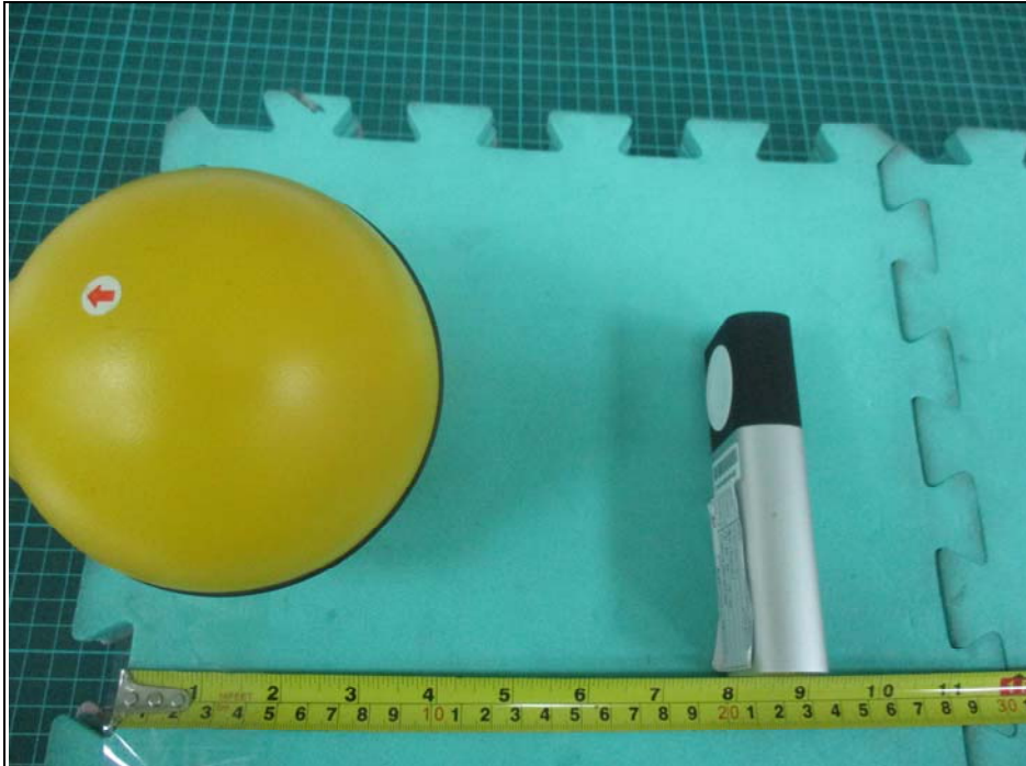
H-Field (Z-axis) (Standby Mode) 20cm
