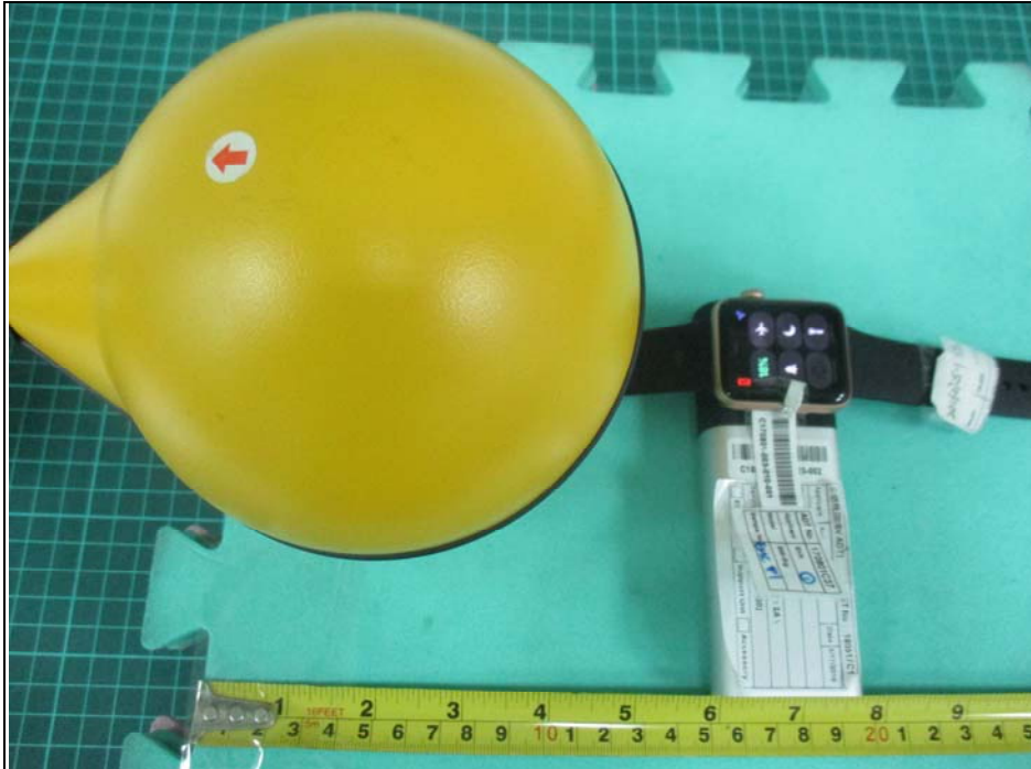
H-Field (Right) (Charging Mode) 15cm
