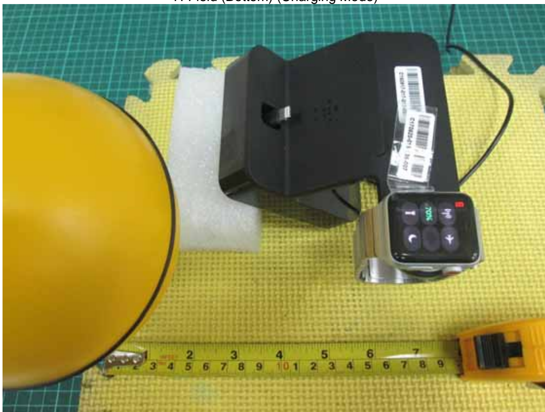
H-Field (Bottom) (Charging Mode)
