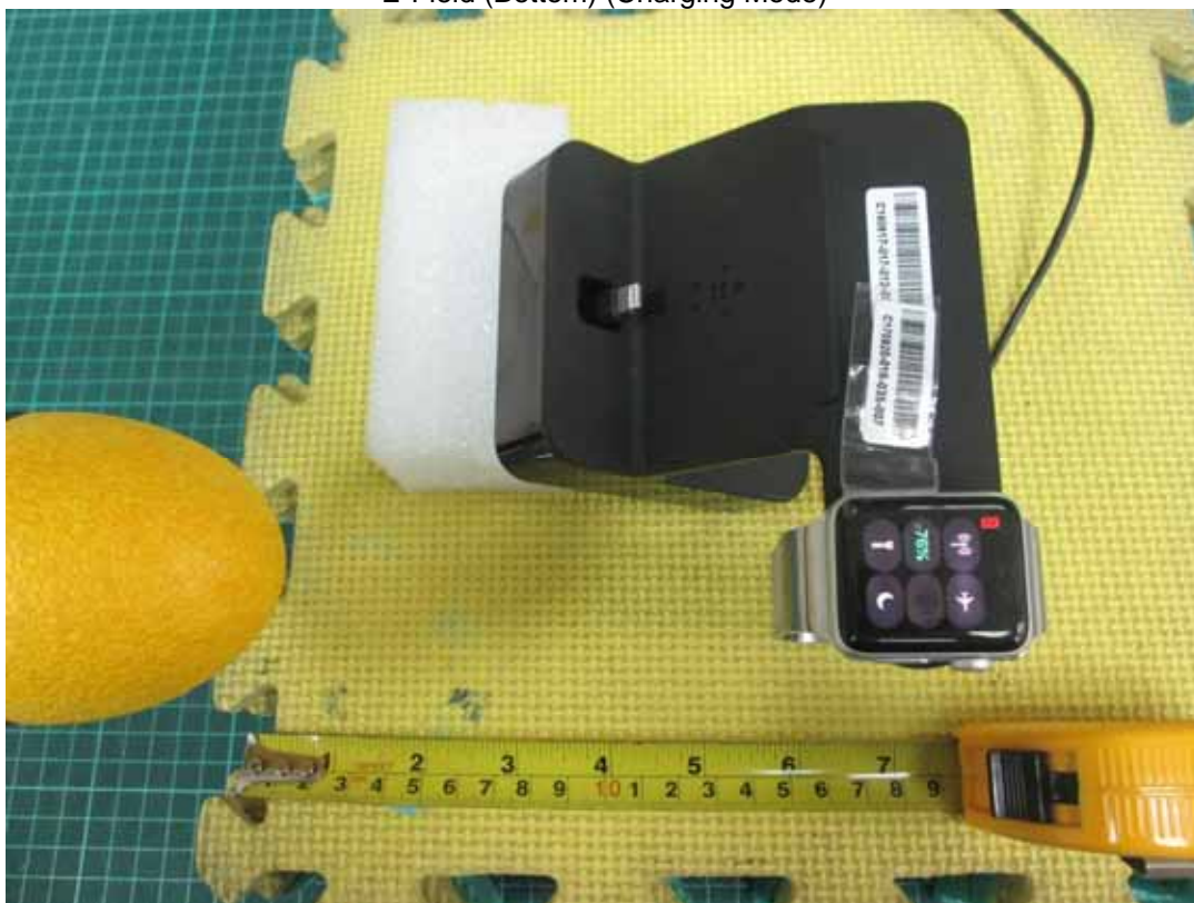
E-Field (Bottom) (Charging Mode)
