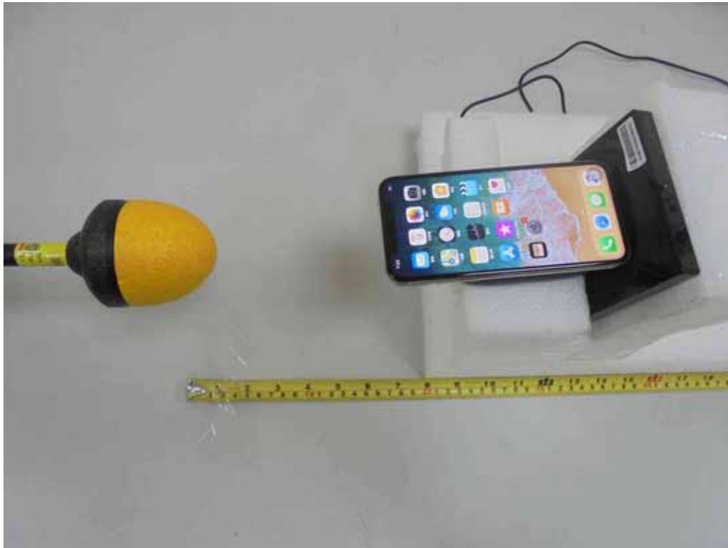
E-Field (Charging Mode (iPhone in the stand-up position) - Z-axis)
