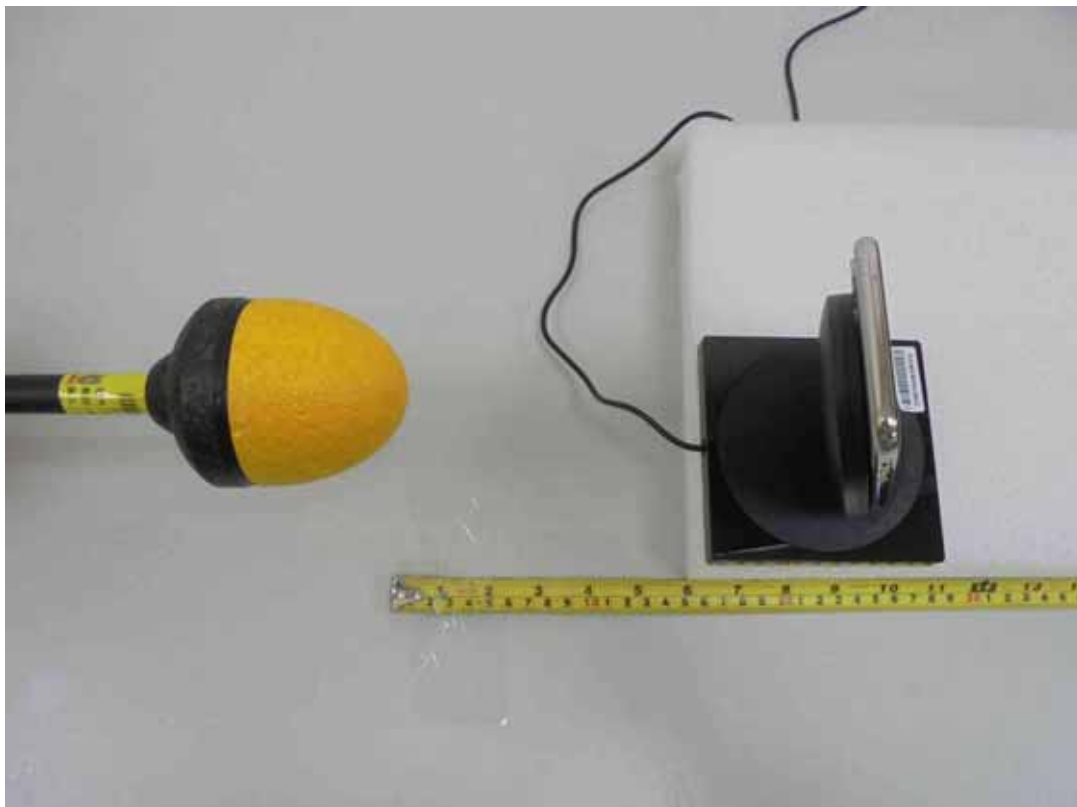
E-Field (Charging Mode (iPhone in the stand-up position) - Bottom)
