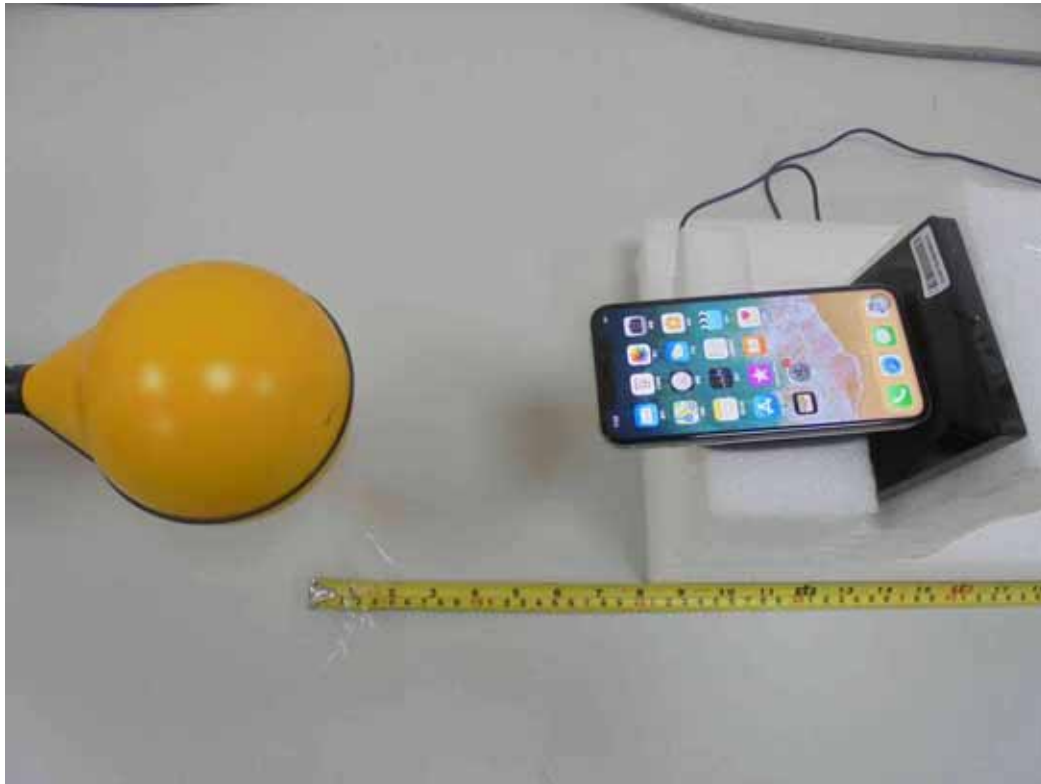
H-Field (Charging Mode (iPhone in the stand-up position) - Z-axis)
