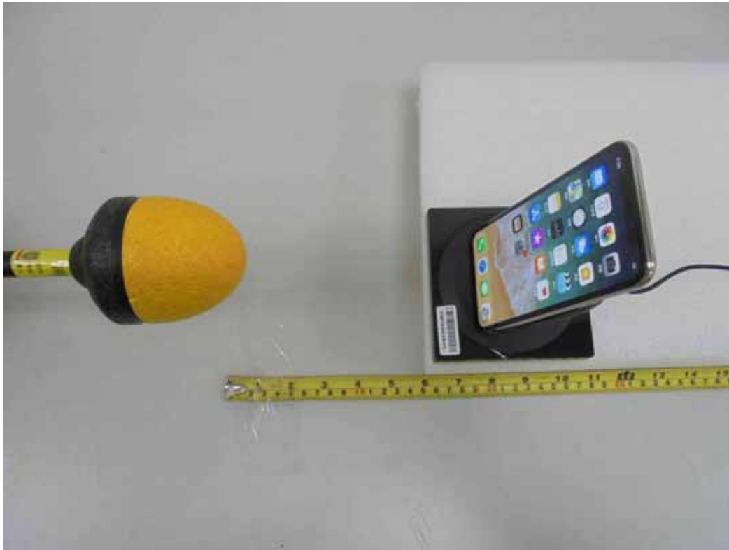
E-Field (Charging Mode (iPhone in the stand-up position) - Top)
