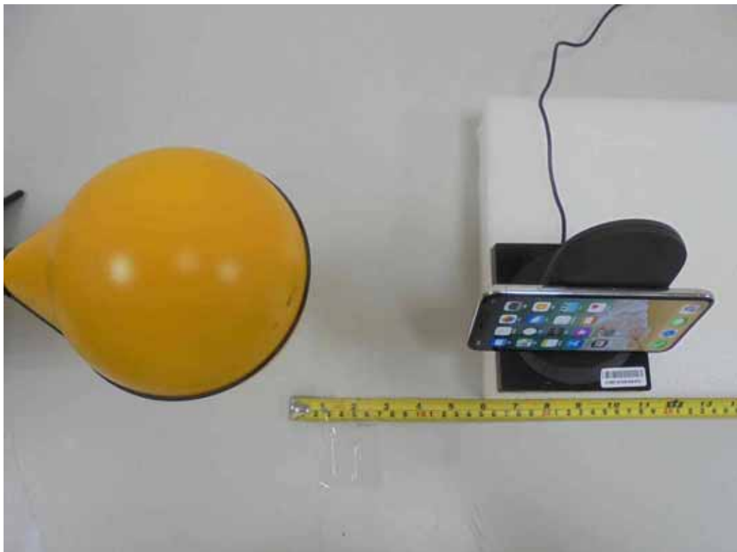
H-Field (Charging Mode (iPhone in the lie-down position) - Left)
