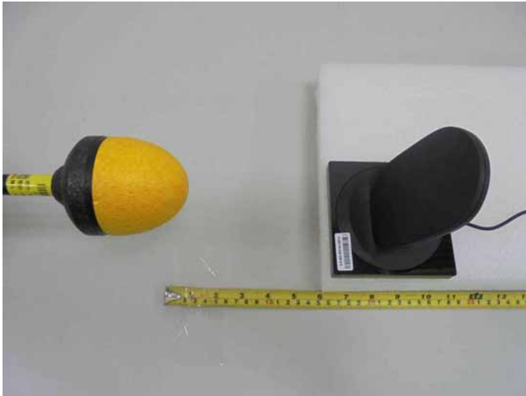
E-Field (Standby Mode - Top)
