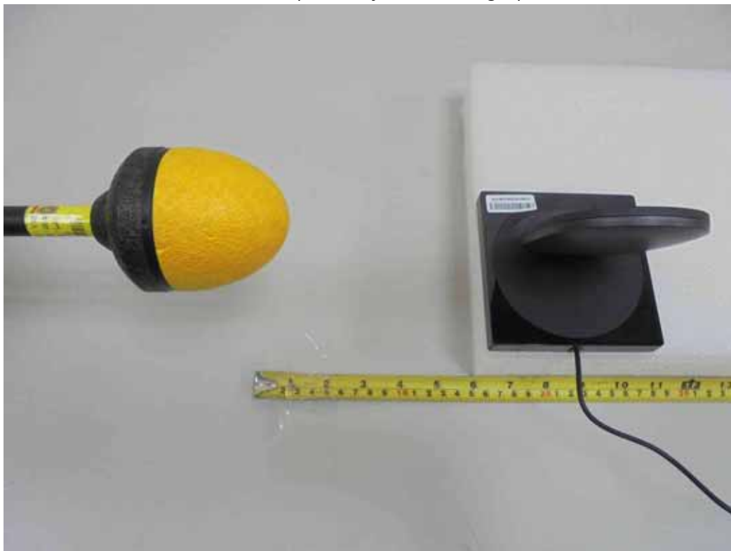
E-Field (Standby Mode - Right)
