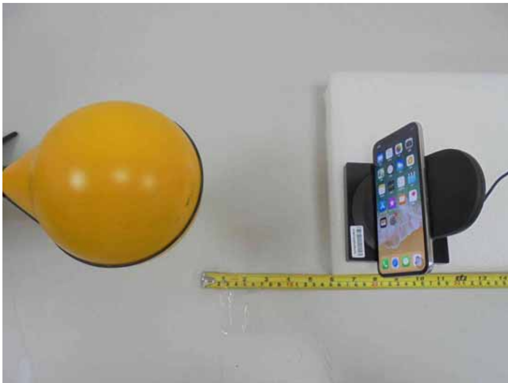
H-Field (Charging Mode (iPhone in the lie-down position) - Top)
