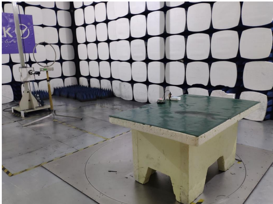
Photos of Radiation Emission Measurement
