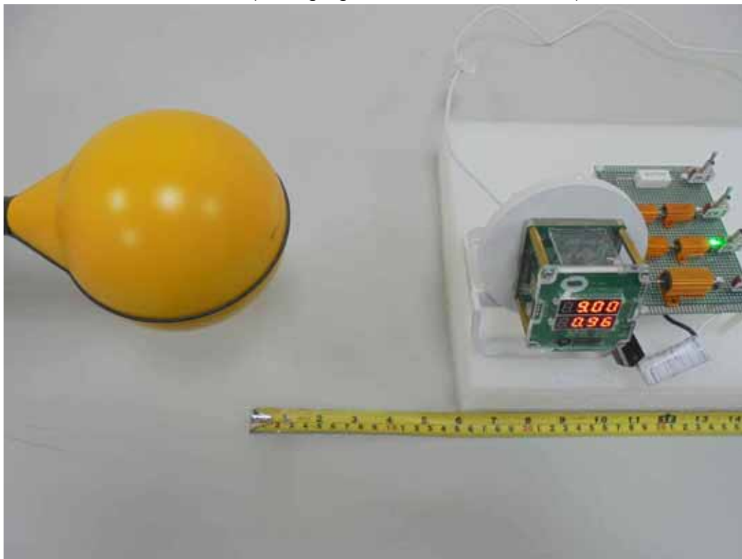
H-Field (Charging Mode with Load - Left)
